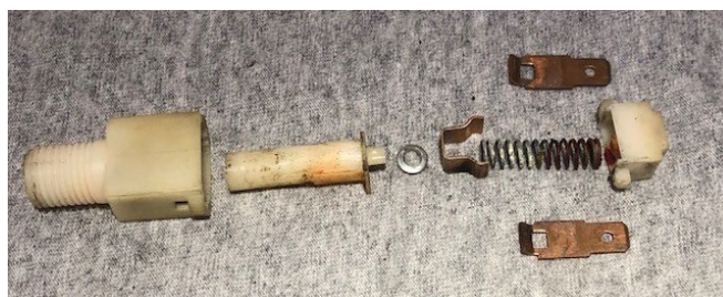
The guts of a TR7 brake switch - now you know.
