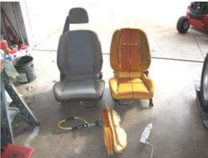
Original Honda Civic seat on left and my 2" narrowed version on the right sans headrest. Alignment on floor pan is near perfect...just hope there is sufficient steering wheel clearance.
