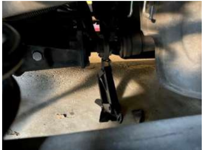
I used a spare TR7 jack under the input flange to rotate the axle into position
