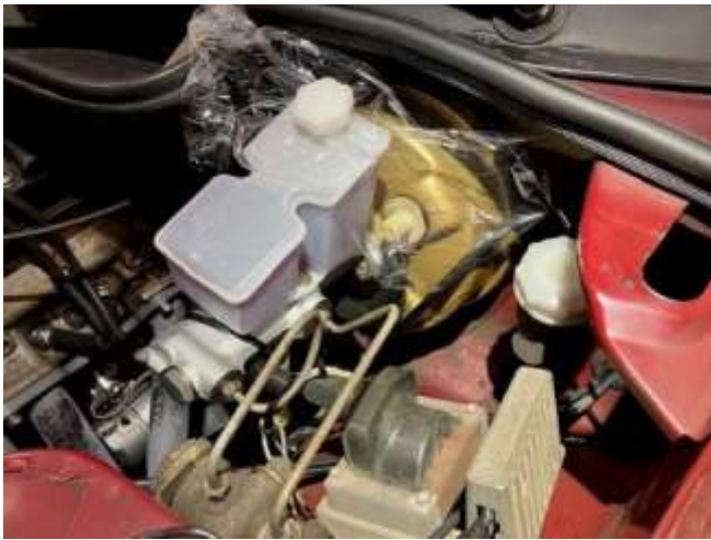
Plastic food wrap under the reservoir cap
