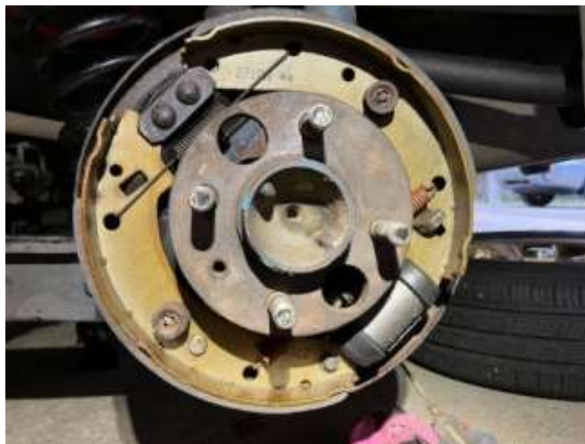
Left side rear brakes after cylinder swap – no big difference from last photo since the cylinders are the same exterior size and shape
