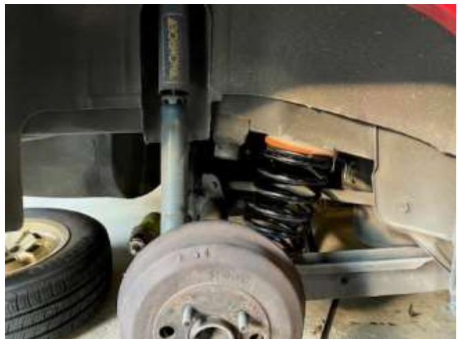
The springs are now new – rejoice! Don't know if it fixed the problem, but hey, progress...
