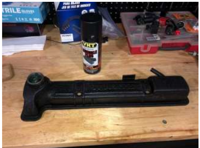
New wrinkle paint on old valve cover – better!
