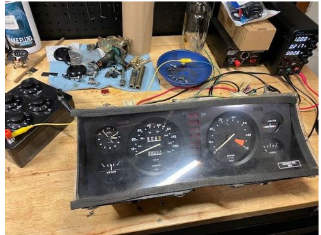
Inca's temp gauge under test with the gauges in the instrument cluster.
