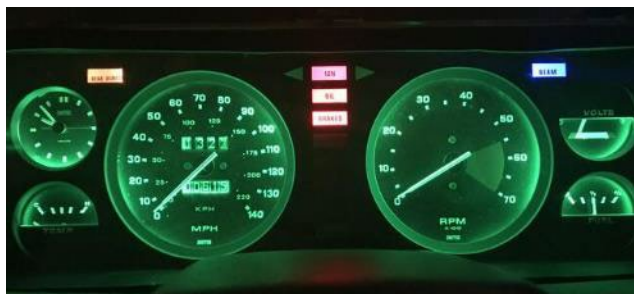
Green instrument illumination showing loss of temp gauge red warning zone color feedback. Hey, look at the IGN light...
