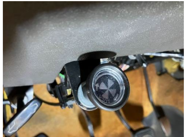
Choke cable installed.
