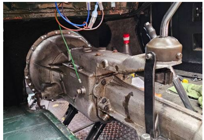
TR4 Trannie with oil leak at the shifting rods
