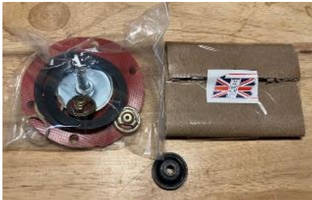
TRF Fuel Pump Rebuild Kit – now with the Oil Seal (at bottom)
