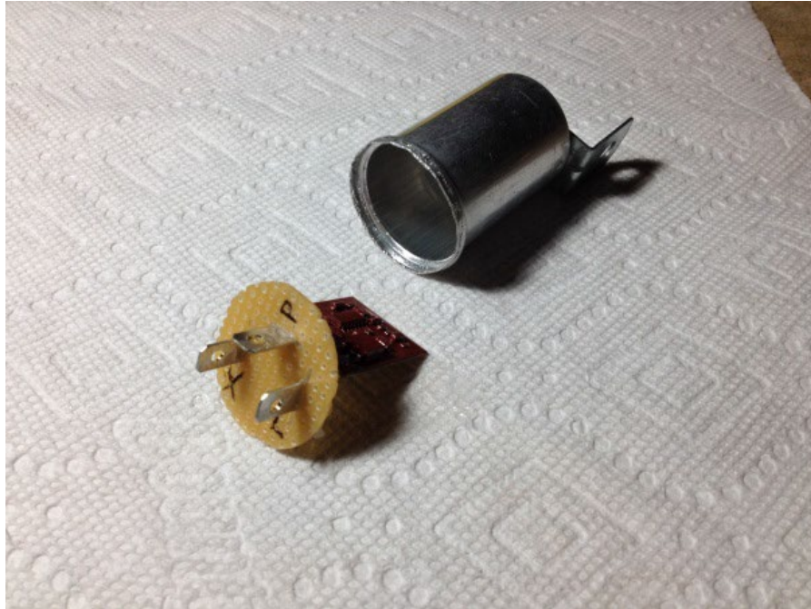
Figure 4 – Circuit board from electronic flasher being readied to put into original-style flasher canister
