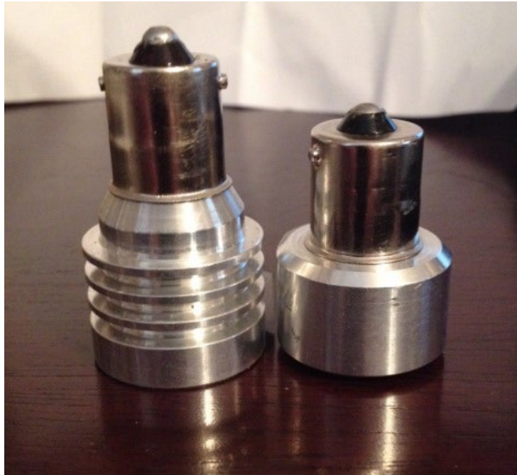
Figure 2 – Difference between the standard LED designed to fit a 1156 socket (and with a dual filament the 1157) on the left and the shorter one required for turn signal applications on my TR3A
