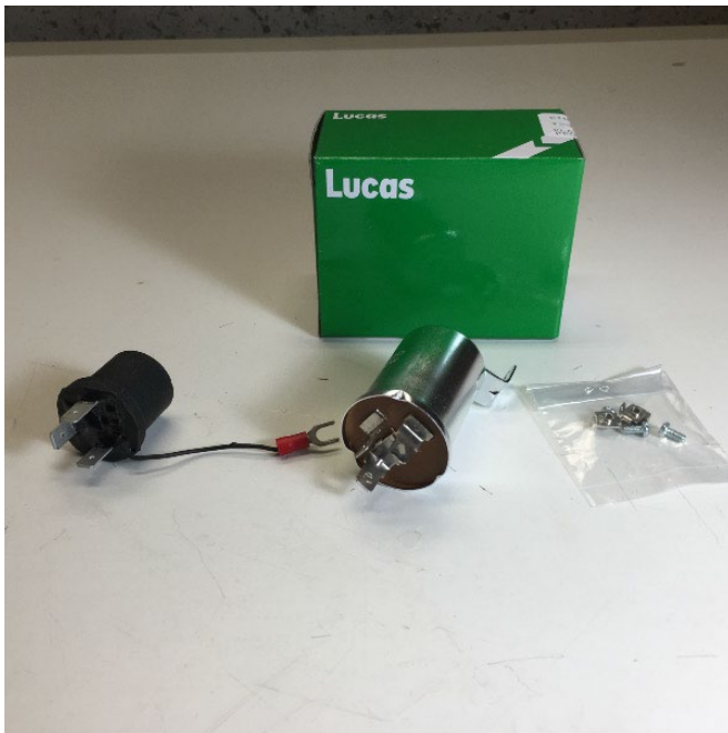
Figure 2 – Donor Lucas can and LiteZupp electronic flasher (left) and Electronic Flasher Unit from SuperbrightLEDs.com (right)
