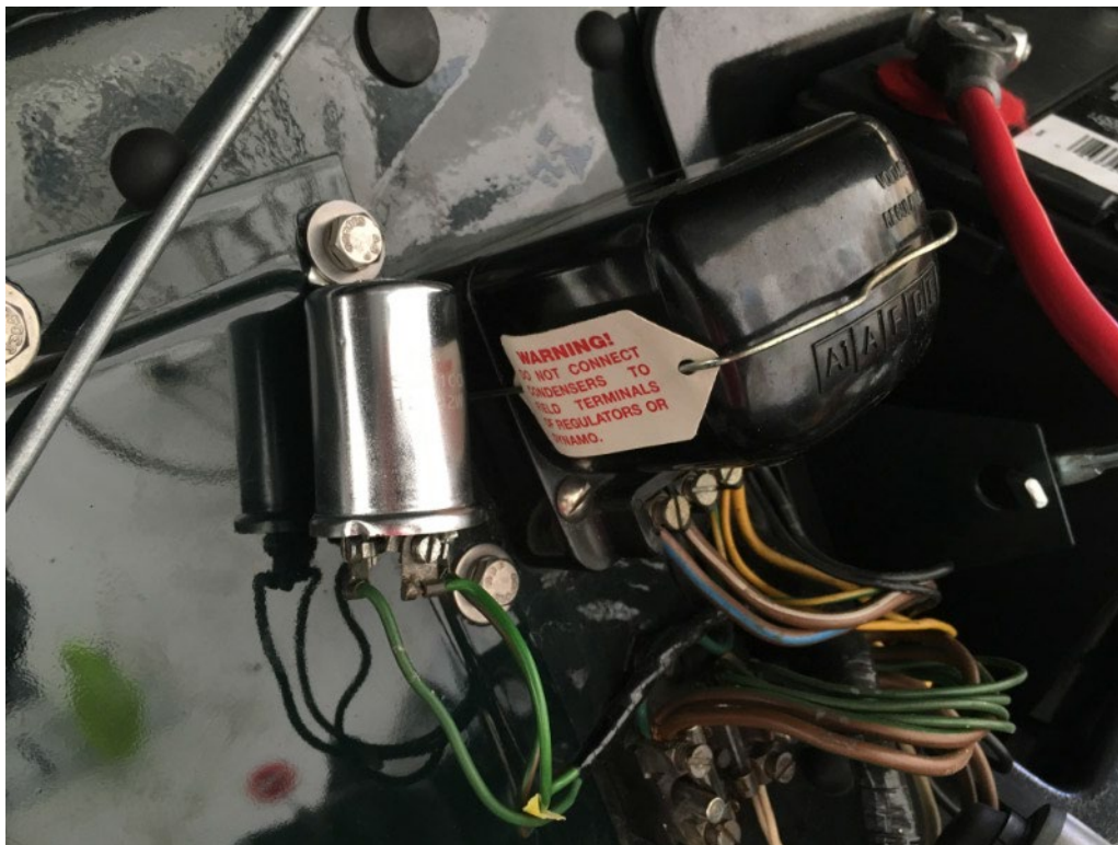
Figure 7 – Electronic Flasher in place in my car
