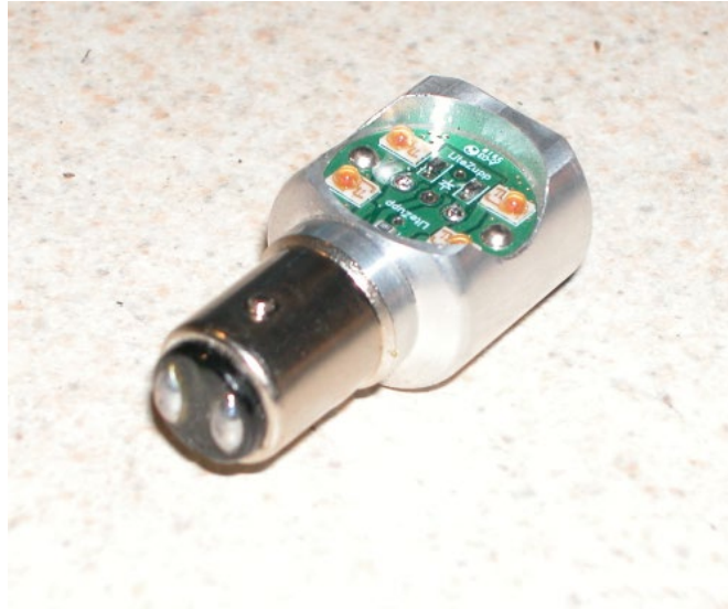
Figure 1 – LiteZupp Red, Right Angle 1157 Replacement LEB Bulb
