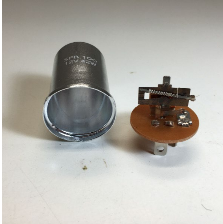
Figure 3 – Yep, that’s all that is inside the original-style flasher
