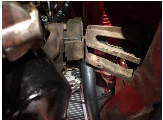
Gap between the bracket and rubber mount shows the space to be made up to get the engine vertical
