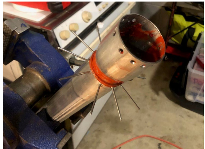
Fun with gobs of pop rivets and sealant
