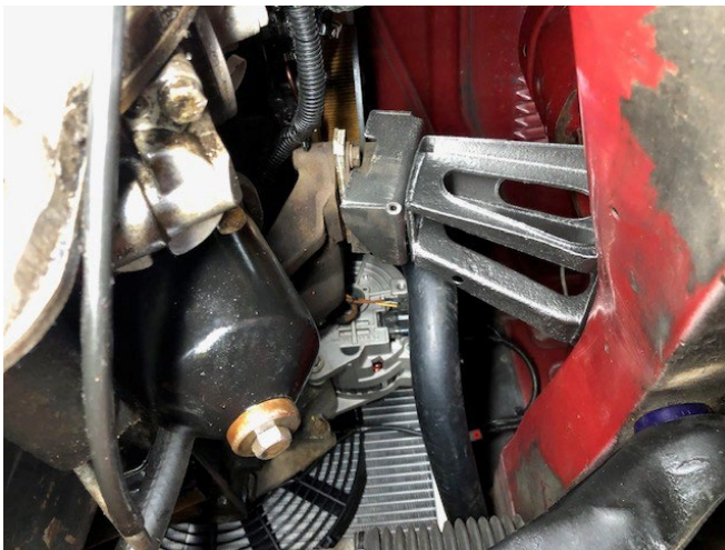
Cleaned-up old mount in place with shims
