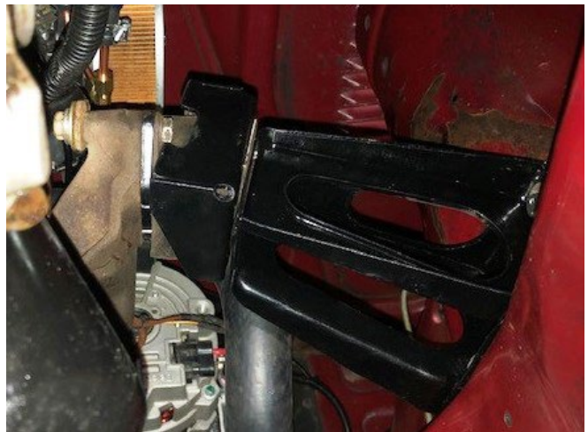
New bracket in place with the shimmed motor mount.
