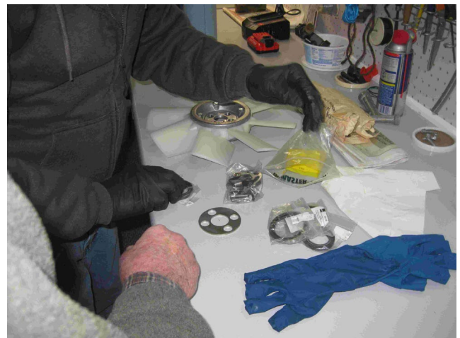
New fan attachment hardware and new fan
