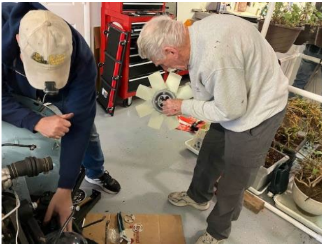
Roger putting the mounting hardware on the new Hurricane Fan
