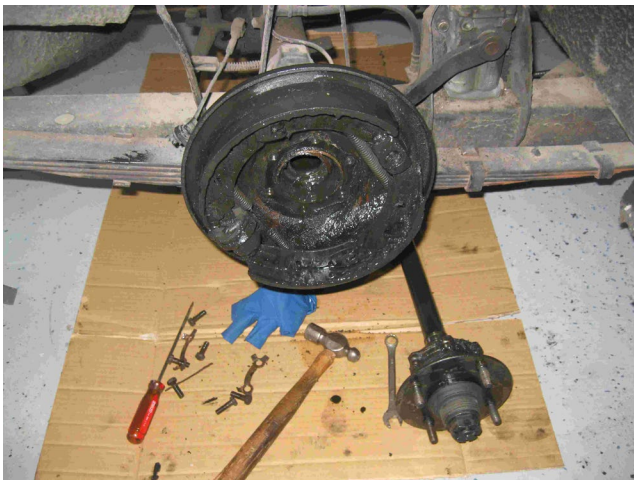
Half-shaft and hub assembly removed
