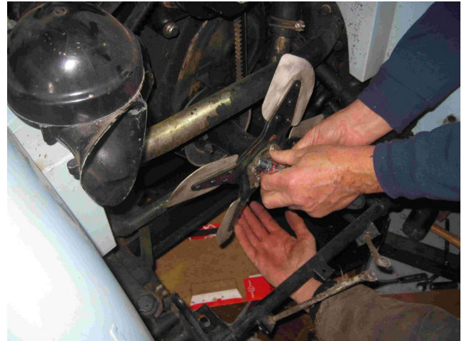
Finally, the nose was off, the radiator removed, and time to remove the pathetic, spatula-shaped fan.
