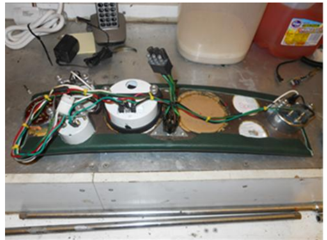
New dash instrument cluster being wired up – note I was still using the original wood one covered with vinyl.
