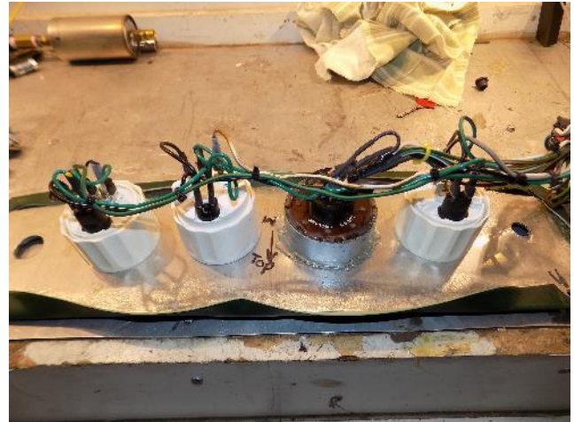
Backside view of the updated instrument cluster using a aluminum sheet to mount them in. This actually was a shot when I went to replace it since the contact adhesive was letting go along the edges...
