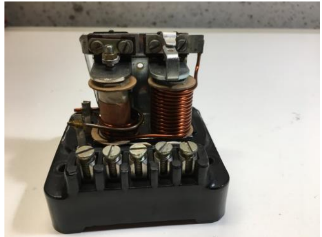
Original Control Box – side view
