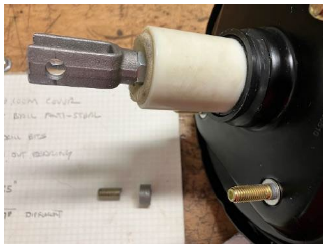
New yoke affixed to shortened servo input shaft
