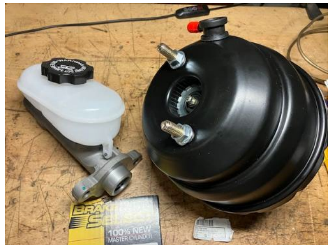
New master cylinder and servo
