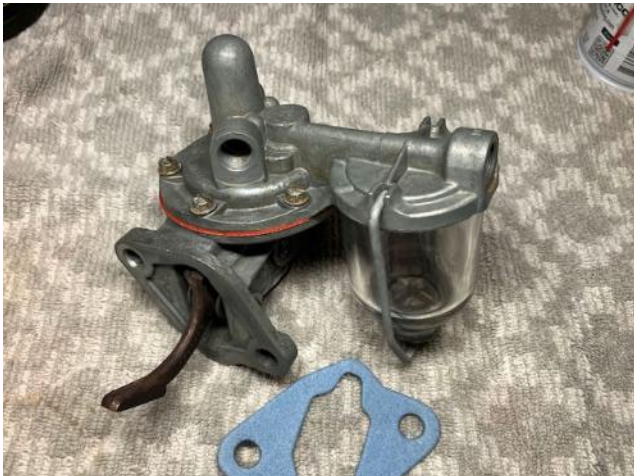
Rebuilt original AC pump, with new gasket, ready to go on a car.
