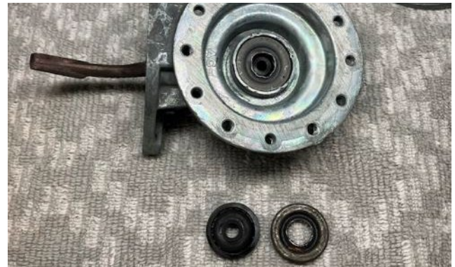
New seal installed in pump housing – below the pump is the old seal (left) and an example of the retainer (right).
