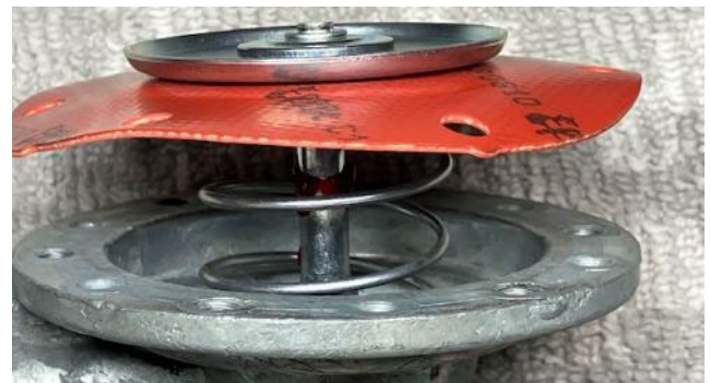
Diaphragm, spring, and rod pushed into the oil seal.
