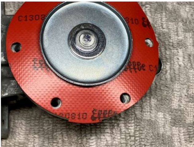
Tab rotated 90 degrees, properly engaged in actuation lever slot – note the holes line up.
