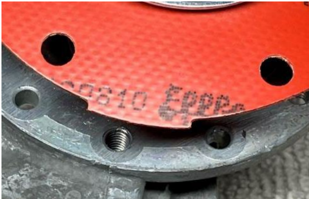
Tab in diaphragm – note holes do not line up.
