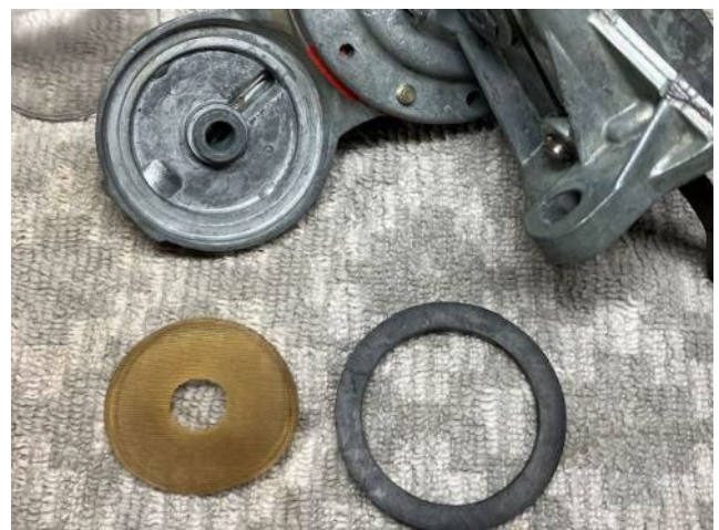
Pump housing, old gauze filter, new seal.
