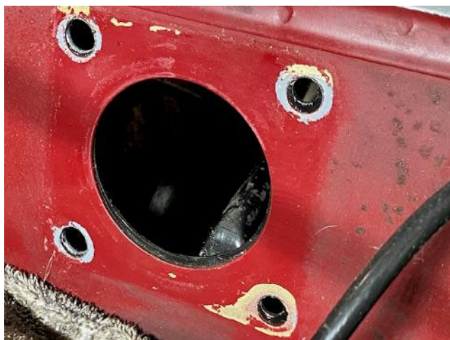
Servo holes in firewall – holes on the left have already been redrilled, holes on the right are stock.
