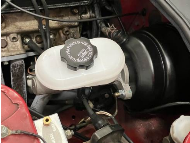
Master cylinder in place to make the lines to the TWS block
