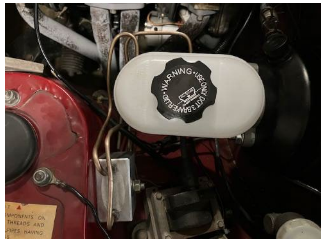
New lines viewed from the top
