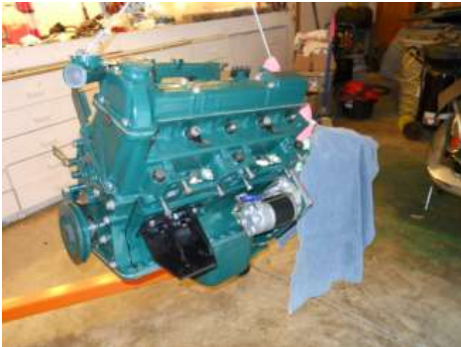
One green engine. Note the motor mount and one of Ted Schumacher's starters. Beach towel is the protect paint as the trannie goes in tunnel
