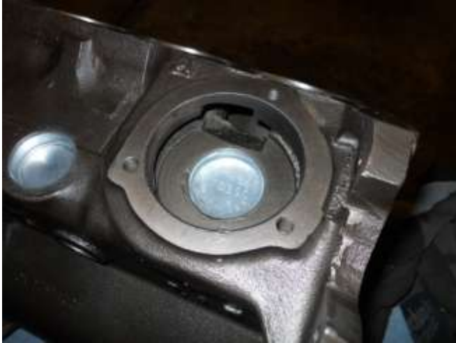
Blocked-off water pump drive hole – there's another plug under this one that blocks the hole to the inside of the engine block, so one plug get's water, the other, oil.
