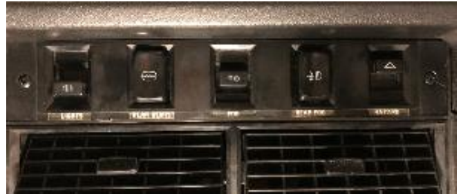
Figure 1 – TR7 FHC Switch Panel
