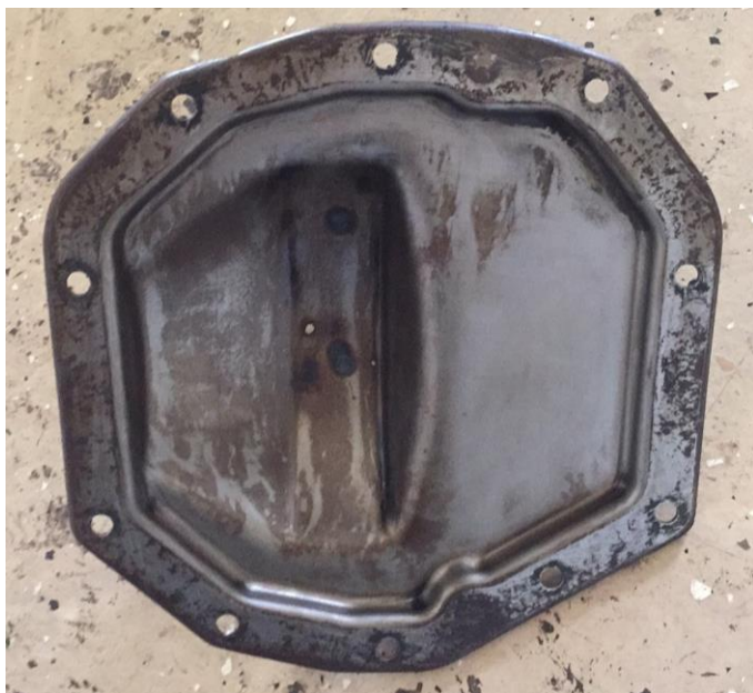
Differential cover with two small holes in the center
