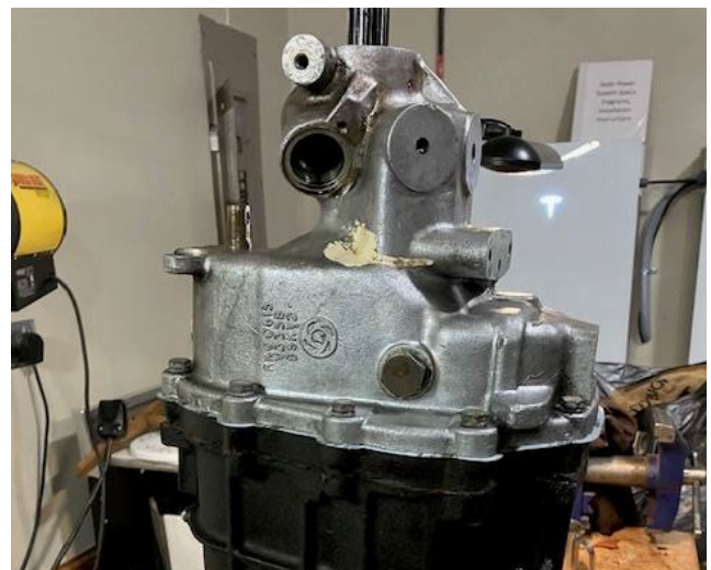
Rear cover in place, bolts tightened. Note the white paint splotch on it.
