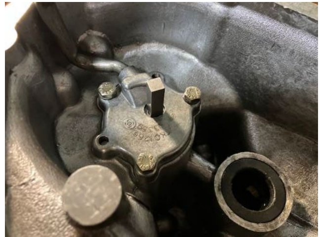
Shaft drive for the oil pump – this was spun around to ensure the pump worked.
