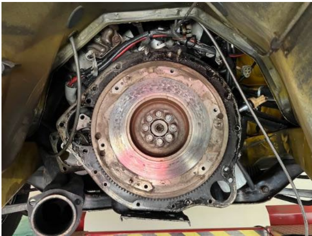
View of flywheel with clutch off – some light checking on the contact surface.
