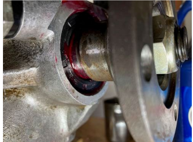
Seal is sealing? Don't worry – that is rubber grease on the seal...
