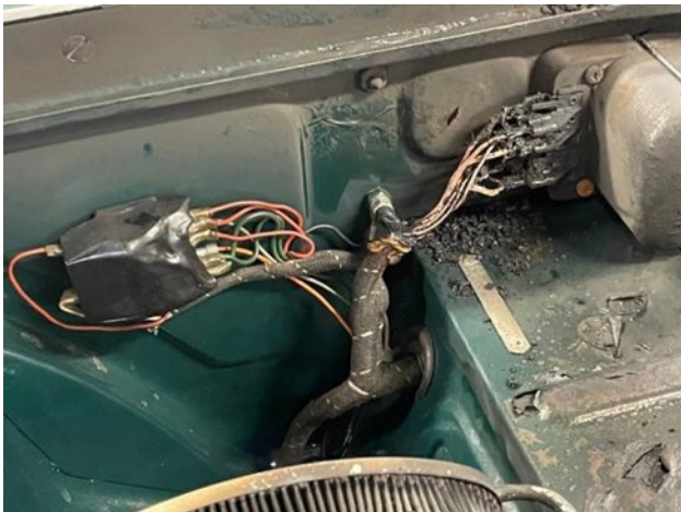
Melted Inner Fender Wiring
