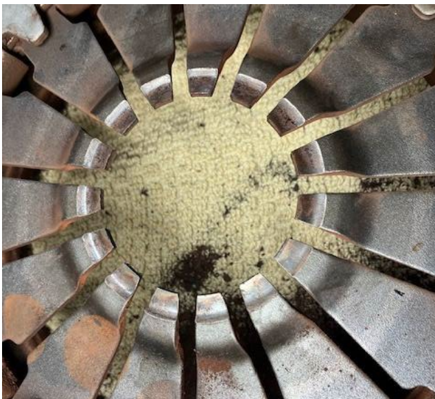
Severe wear on the tips of the fingers due to contact with the release bearing
