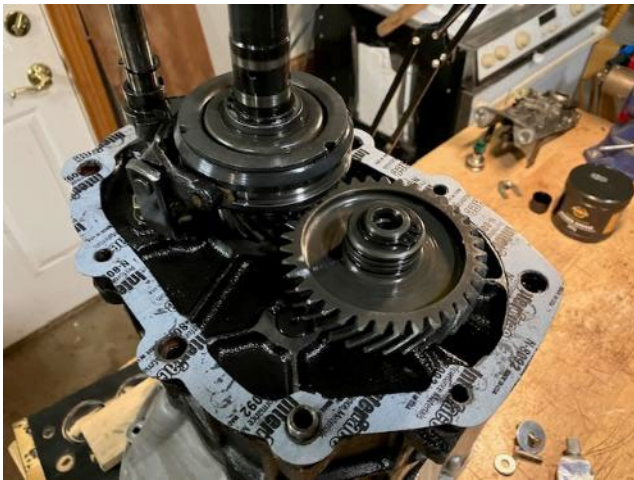
New gasket in place for the rear cover.
