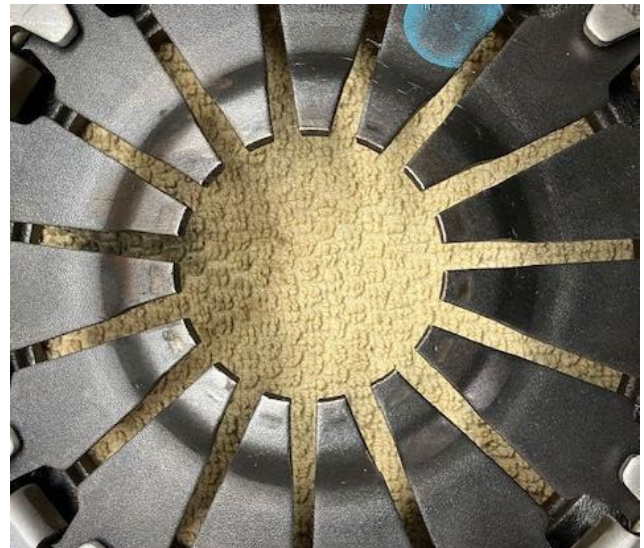
Used pressure plate assembly with very light wear evident
