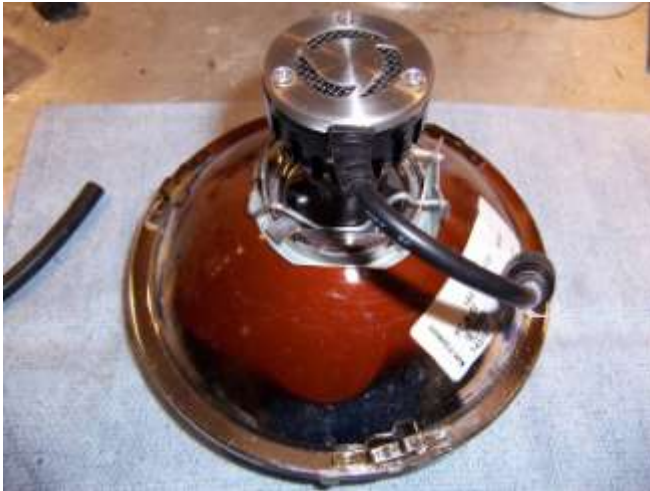
LED headlamp bulb in Hella Stag Headlight Lens
