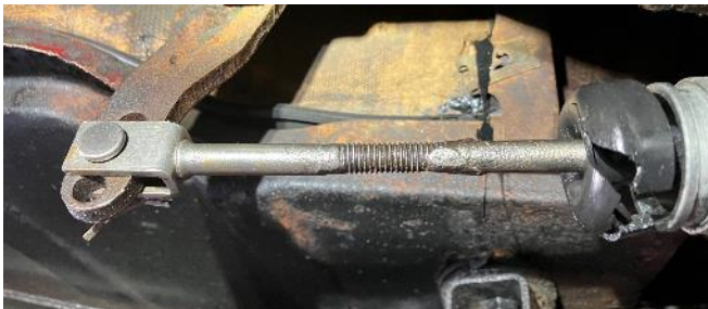
Clutch actuation rod – the Frankenrod!
