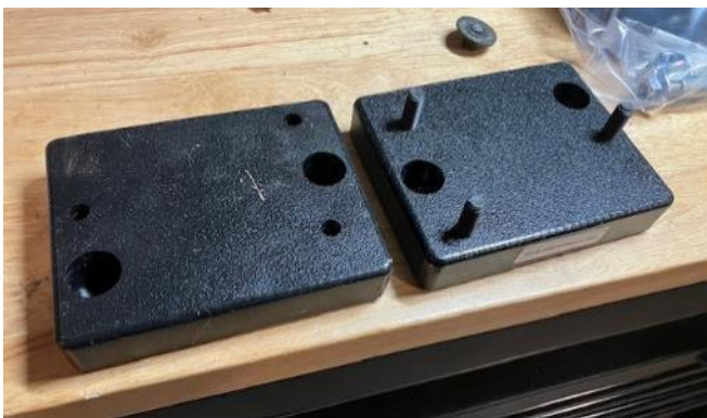
New spacers – made of solid plastic. They came with bolts already in the holes I needed to use for the captured studs in the bumper. Knocked them out and drilled out the holes a
