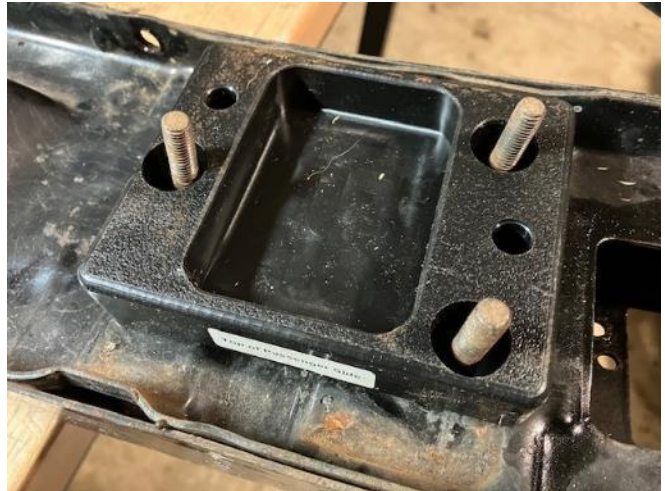
Trial fit of the new plastic spacers to the bumper – fits fine, okay, after I drilled out the holes a bit, fits fine...
