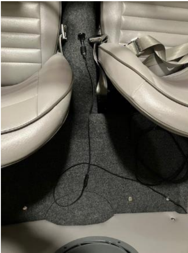
The switch in place between the seats – sticks right to the top of the drive shaft tunnel
