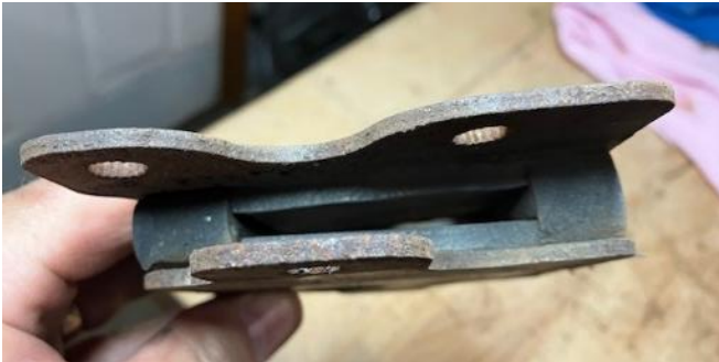
Edge on view of the spacer showing the rubber middle – left is the top, right the bottom – you can see that the plates are no longer parallel – top was in compression and bottom in tension due to weight distribution of bumper. Not as evident here is the sag, it did.
