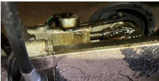
The source of the transmission leak – O-ring seals in the shifting fork rods
