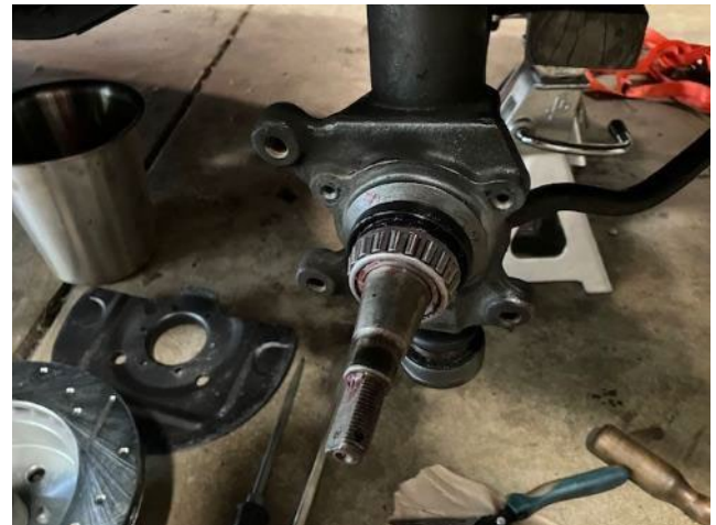
Well, isn’t this a dream...Inner bearing stuck on the stub axle.
