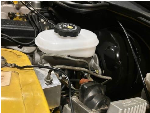
New master in place on the new servo
