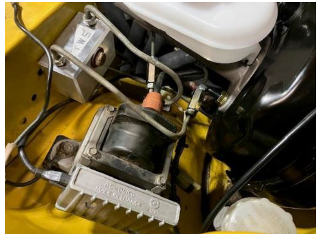
Funky tube bends to clear the coil – the “Frankenlines” – you can see the line connectors just above the coil in this photo.
