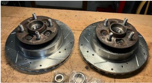
New front rotors on the hubs – vented, cross-drilled and slotted.
