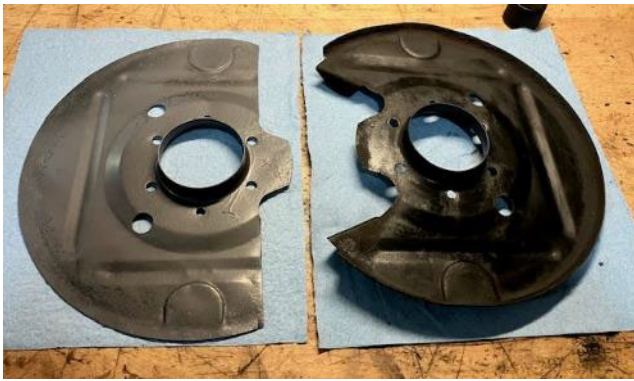
Front Brake Dust Covers – modified on the left, stock on the right. Yes, that’s a Ford gray metallic paint, so sue me...
