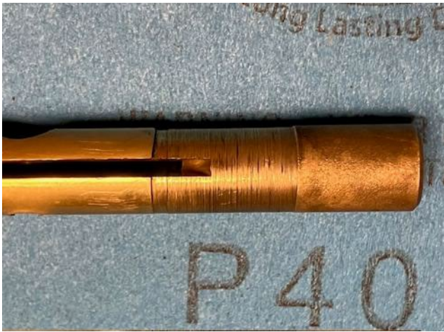
Visible wear on throttle shaft, about what you would expect for a carb that has maybe 80-90K miles on it...
