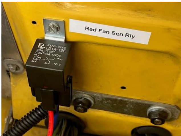
Updated sockets for the Radiator Fan Sensor Relay
