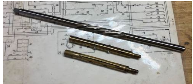
0.01" Oversize ream on top. 0.01" oversized shaft in the middle, working original on the bottom.
