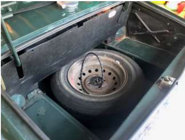
Solid car – note the remote fill line for spare tire air!
