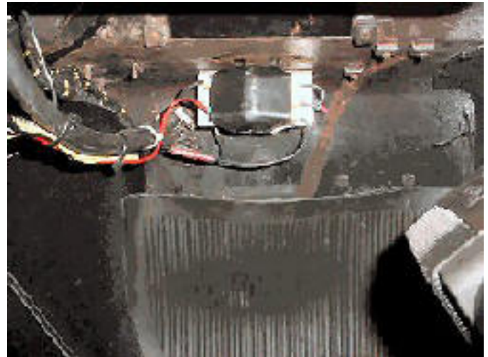
Extra fuse box under the passenger’s firewall. No, it’s not up to John Ewell standards, but few are!
