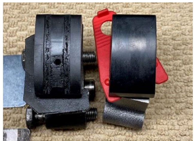
Original shoe on left (showing some wear due to use), new one on right. New one does not have chain oiling hole.
