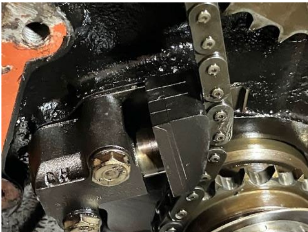
Hydraulic tensioner showing a bit of wear...
