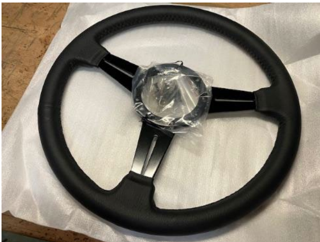
Wheel Moss sent for the TR7 – the center is on the same plane as the rim- it's flat and will not work right.
