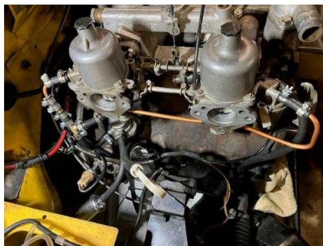
New fuel lines routed
