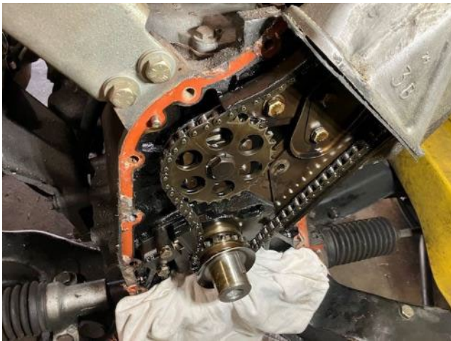
Cover off – looks okay? Note rag at bottom to keep things from falling into the oil pan.
