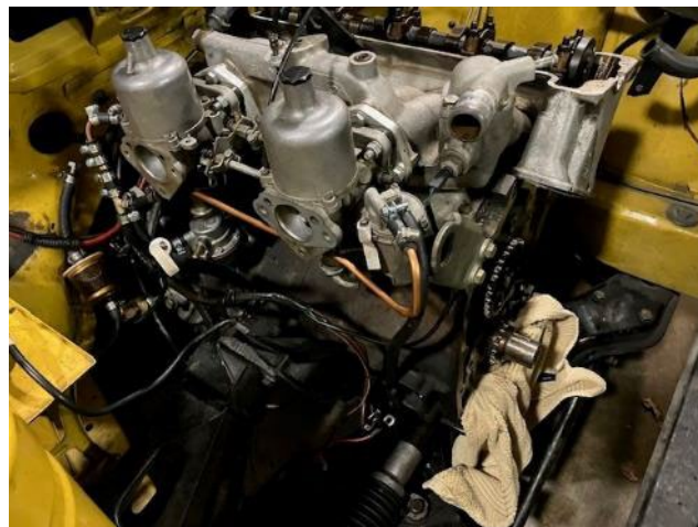
New fuel lines routed
