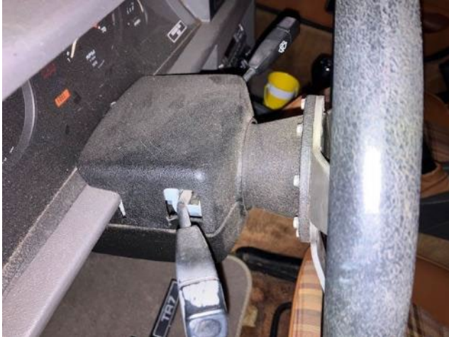
TR7 (and 8) steering wheel – note the offset of the center to allow hands to clear stalks.
