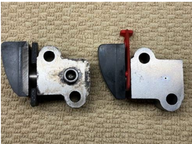
Original tensioner on the left, new on the right
