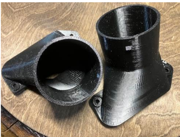
Printed vents as delivered
