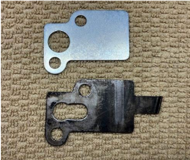
New tensioner backing plate top, original one below.
