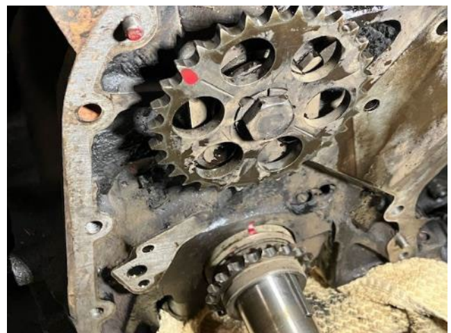
TDC marked on the crank gear and desired distributor location marked on the jackshaft gear. You might note this jackshaft location
