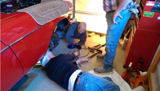
Working on the front springs on the P1800 – much easier than a TR8, or a TR3 for that matter...
