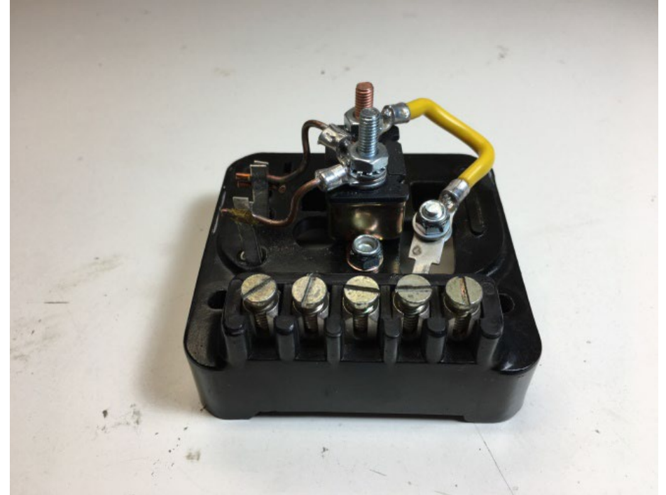
Final empty voltage regulator with fuse
