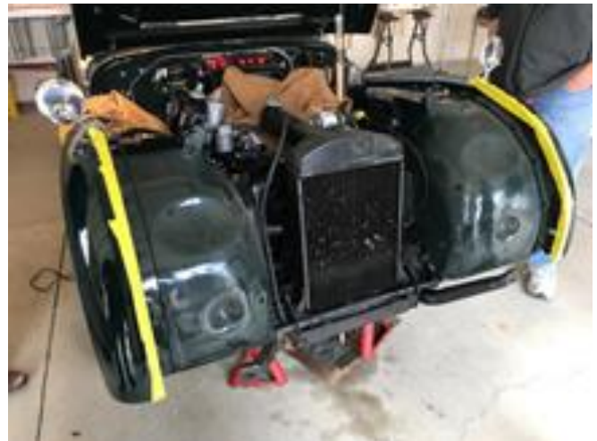
It cools much better without that blocking front shroud...
