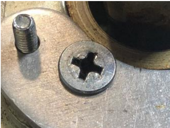
Showing larger screw not fitting flush
