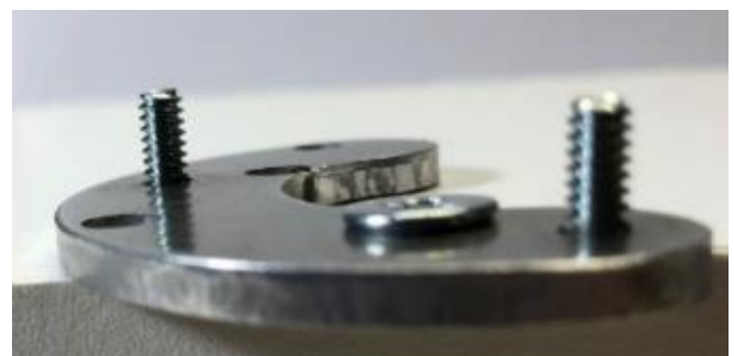
Showing screw in “bad” adaptor
