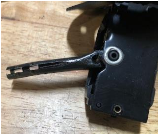
Close-up of arm - the rod goes through a hole in the arm near the pivot and then snaps into a channel in the arm - the plastic had slightly deteriorated allowing the rod to slip out
