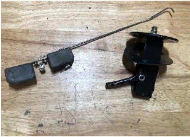
Sender (right) and the rod with floats that fell off (on top and left)
