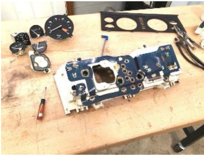
Shot of flex PCB on back of instrument cluster housing - note the gauges have been removed
