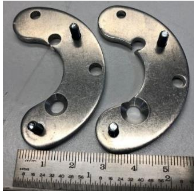
Incorrect adaptor plate on left, correct (old) adaptor plate on right.
