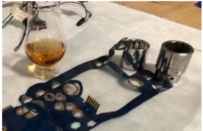
Sockets used to hold (and flex) PCB in place to attached loose traces. Adult Beverages optional.
