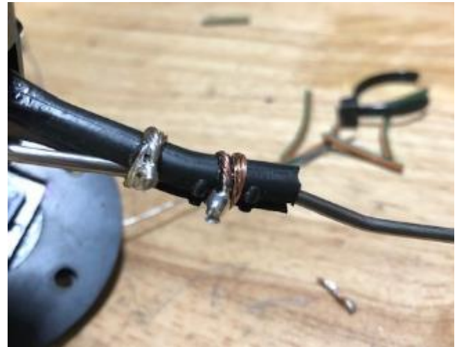
Wrapped copper wire around the arm to secure the rod in two places then soldered the ends to keep them in place
