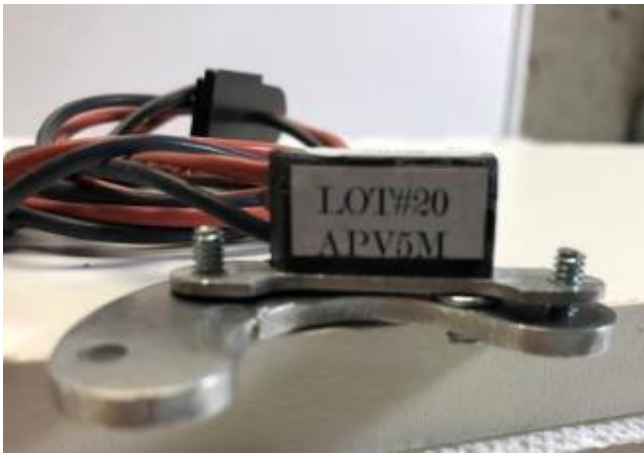
Showing module “cocked” above screw on “bad”
