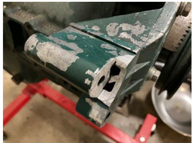
10mm off the alternator bracket where the Min-Denso will mount.
