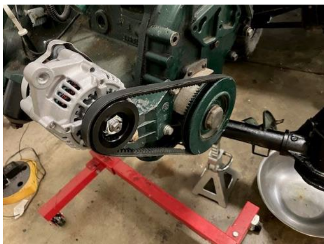
V-belt attachment went well – time to clean-up the bracket and develop the rest of the attachment hardware.
