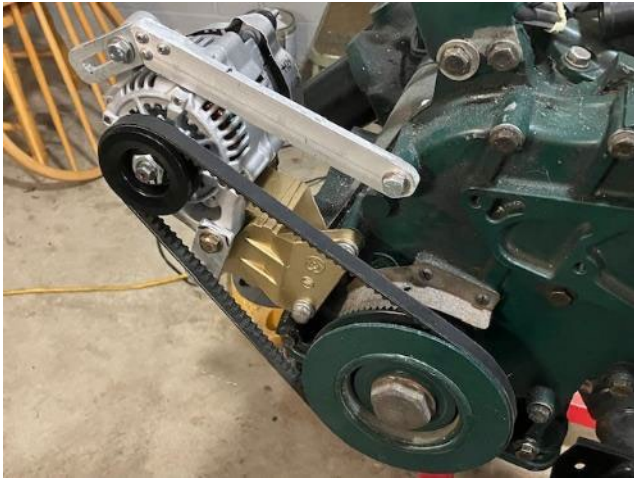
Mechanical connections in place – looks workable if not industrial.
