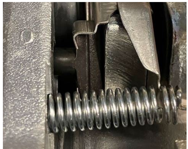
TWS Motors parking brake actuation pin attachment to actuating plate.
