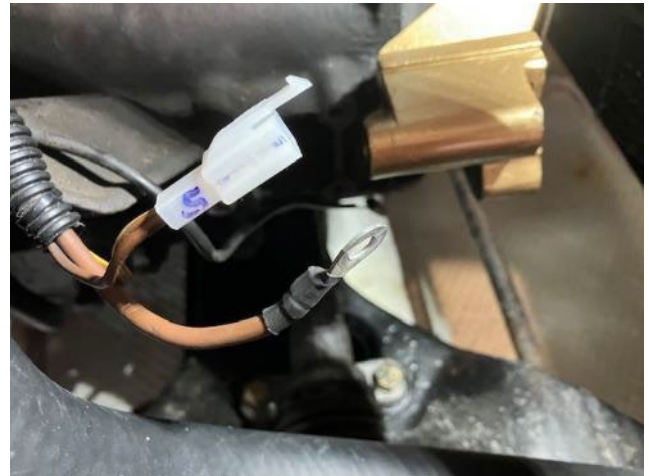
Added an intermediate connector to the alternator connections to make swapping easier.
