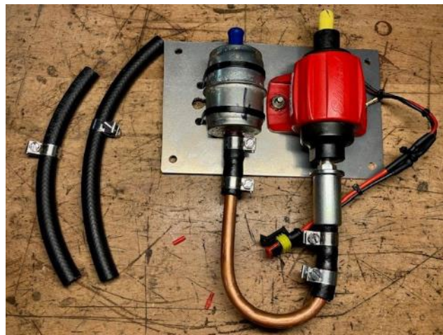
Back-up fuel pump assembly
