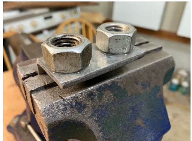
Those large nuts epoxied to the parking brake cable bracket. Follow me for more intuition-based solutions.
