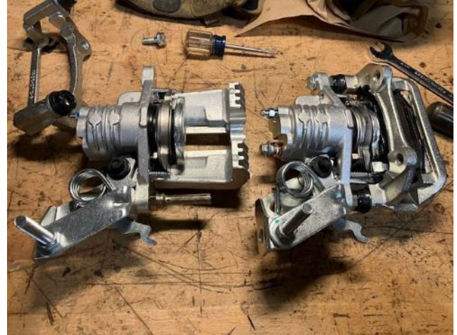
TWS Caliper on the left, O'Reilly one on right – they are the same, but different.
