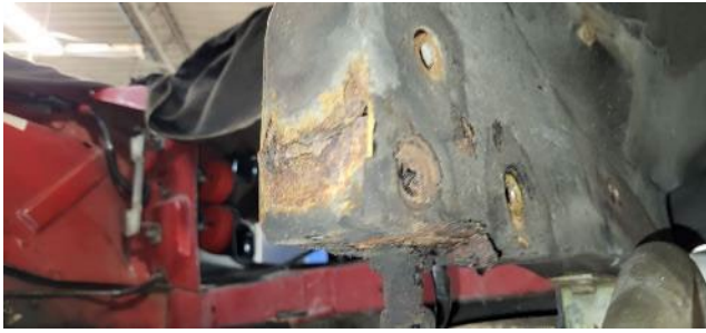
Picture of front rail rust damage.
