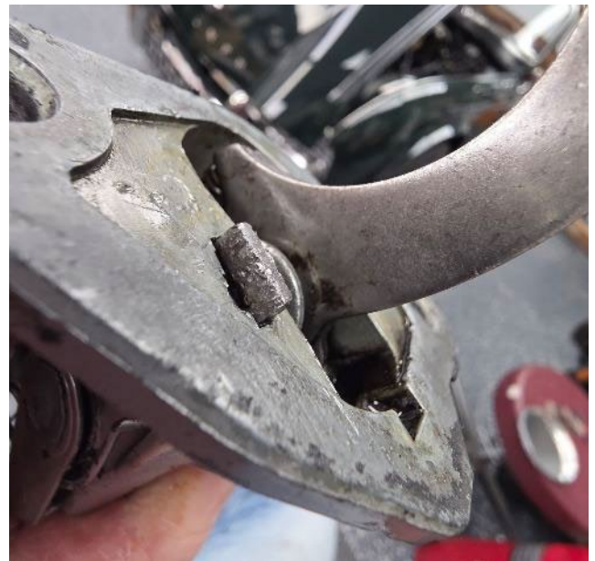
The wedge block that holds the lever pin in had the staked metal that holds it in fail.
