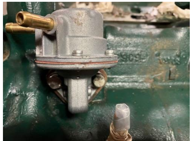
Side-on view of the fuel pump and the two bolts that hold the pump on in the stock configuration. The pipe end covered with plastic to the lower right of the pump is the dipstick pipe, showing the kinda stuff in the way of getting the pump in and out.
