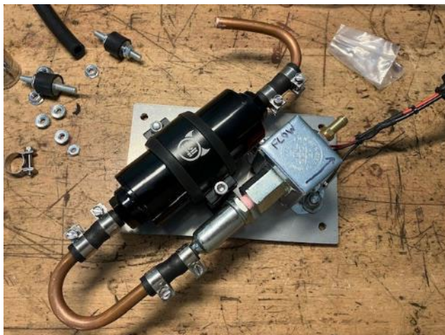
Parts mounted to plate – note the dual-filtration
