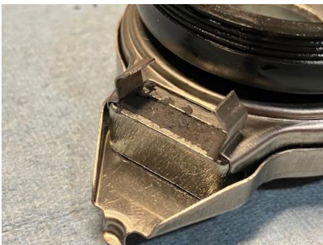
Trench filled in with steel epoxy.
