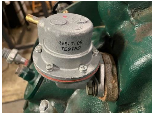
Stock mounting position of late-style fuel pump - using the old FrankenStag TR7 engine as an example. Note the bolt and the spacer.
