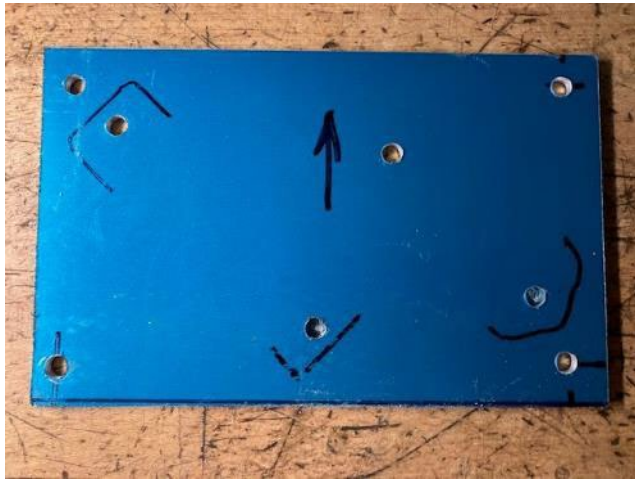
Plate cut and drilled to size
