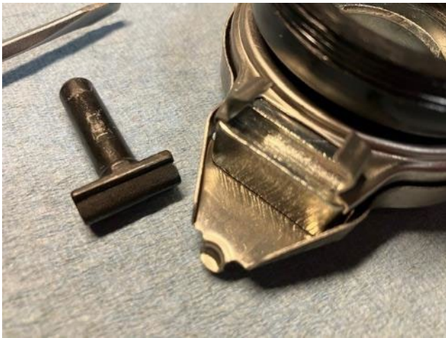
Pin removed showing trench it rides in.
