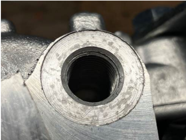
Rough surface on the fluid supply port.
