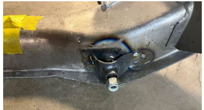
A-Arm repair unpainted.
