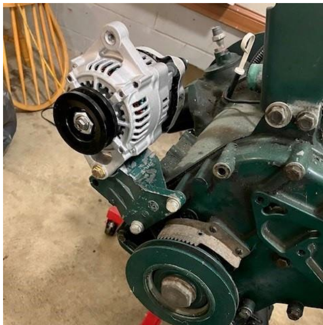
Mini-Denso on the bracket – looks fairly good – time to put on a v-belt...
