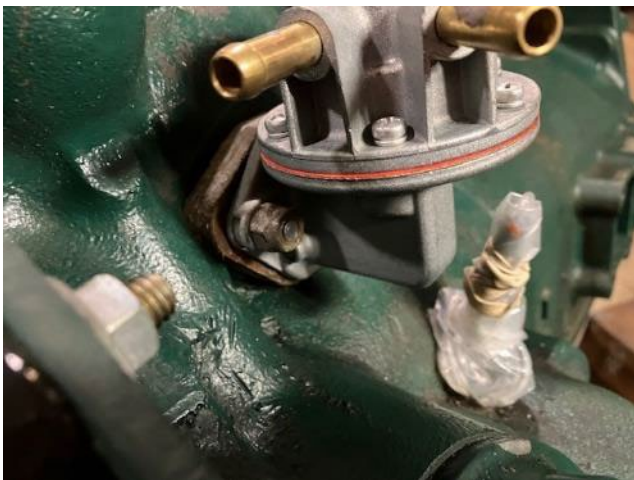
Pump in place using studs and nuts rather than bolts.
