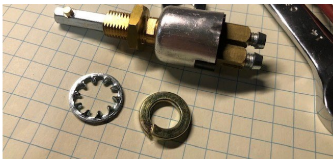
Moss switch, lock washer supplied on the right, the one I used on the left
