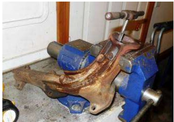
Tapping the drilled-out stud hole...
