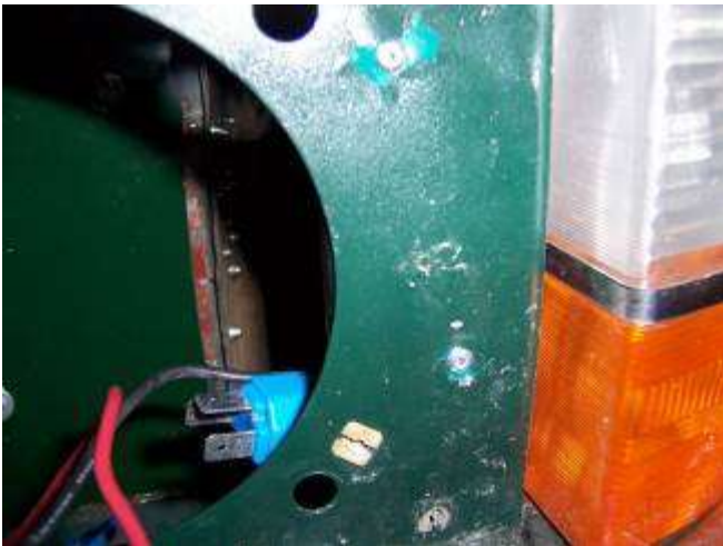
Driver's LED Power Convertor Pop-riveted to back side of the front valence, driver's side. Evidently the paint here wasn't prepped good for that last respray....
