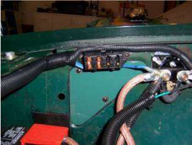
Figure 3: New Fuse Block To Handle The Much Higher Load
