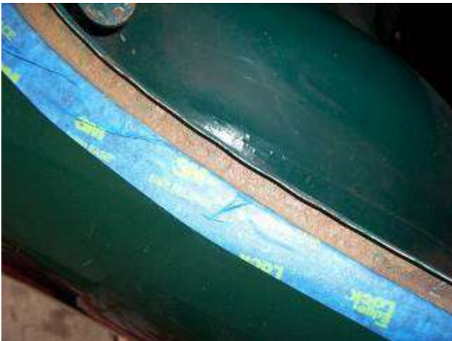
Rust in the targa top seal on the passenger side
