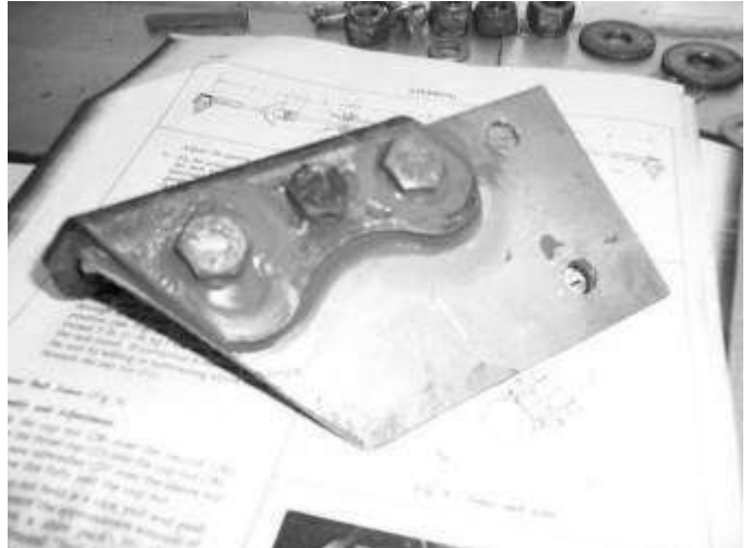
New Driver's Side Bracket Made From The Old Bracket And A Piece Of Thick Rolled Stock.
