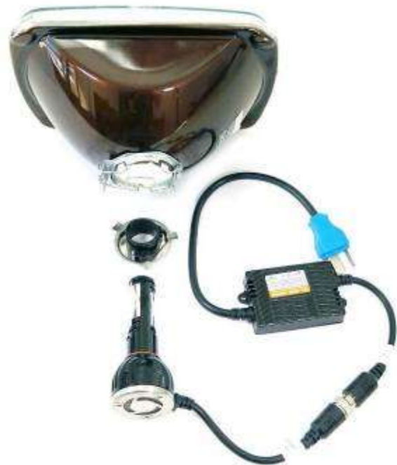
Expanded view of the LED bulb and power conditioning
