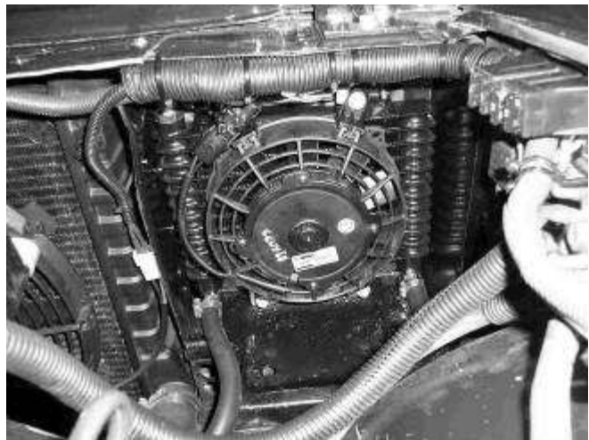
Trannie Cooler Where The Battery Used To Be
