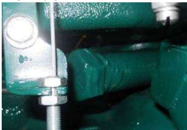
Large bolt, liberally coated with JB Weld epoxy screwed into heater hose port. That will stop the leak – Conan away!
