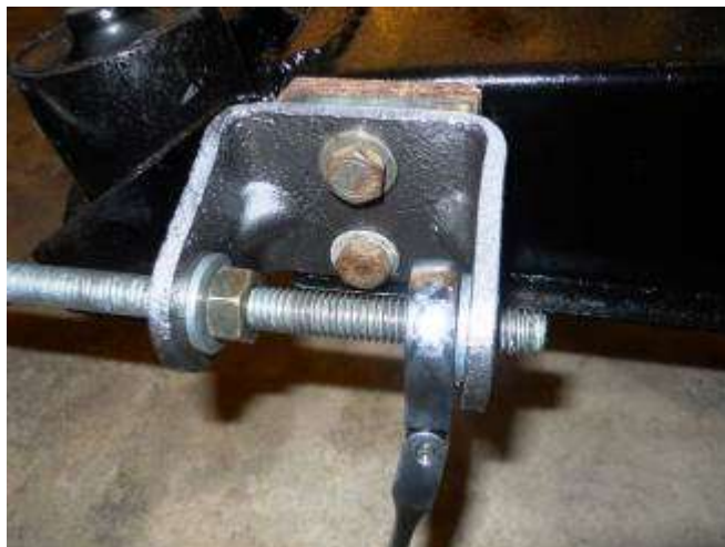
Two-foot rod as an expander tool
