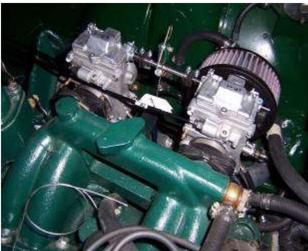
Choke cables in place – note that they have to run forward a ways before you can reverse them due to the intake manifold
