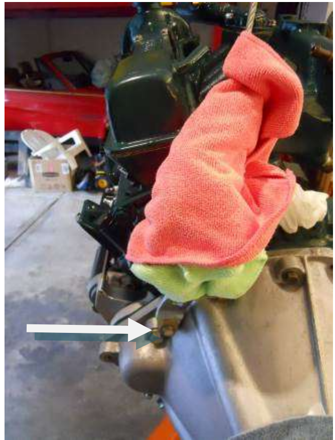
Back lift attachment – used the rags to save block paint job
