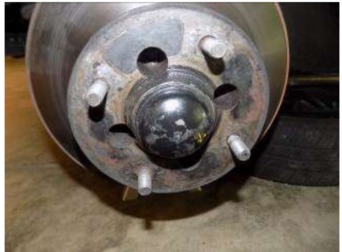
Dust cover back in place
