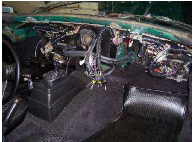
The dash torn apart to get at the wiring harness
