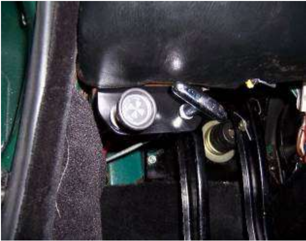
New bracket under the dash where the old bracket was, cables installed
