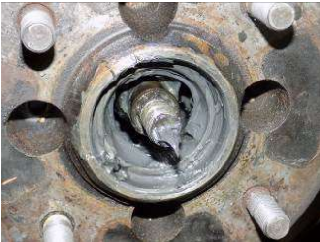
Moly grease laid on to the outer bearing's outer race
