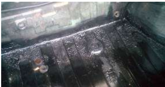
Lifted paint on the FrankenStag trunk floor. Oh, the humanity of it all!
