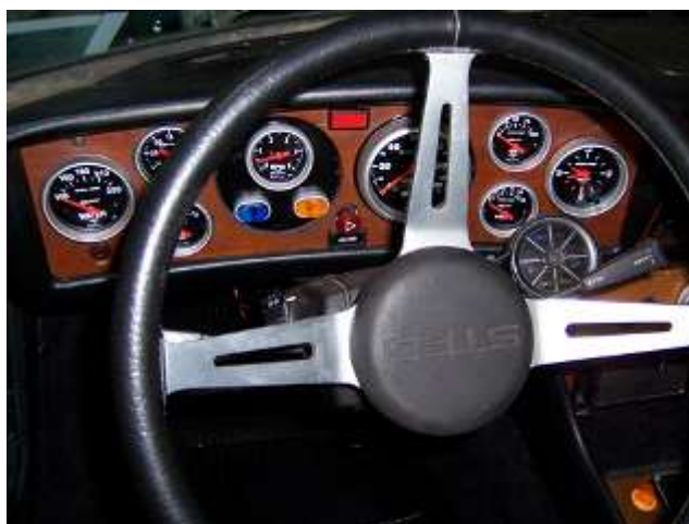
Close-up of dash – note where I put the radiator fan and fog light switches – under a smaller tach where the old tach went.
