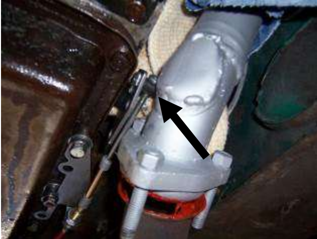
Drat! Shifter Linkage Hits Exhaust Pipe, More News At 11...
