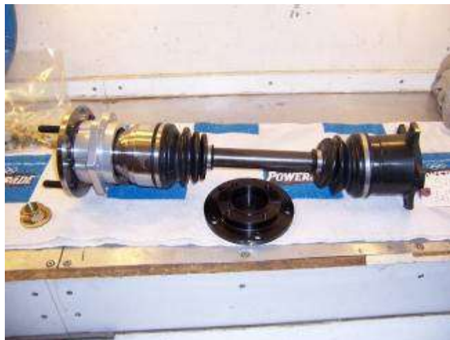
Goodparts Stag Half-shaft – uses CV joints instead of U-joints
