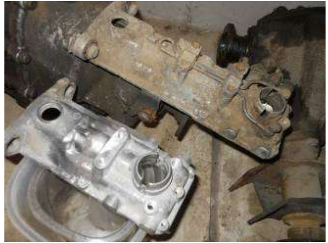
Stock shifting extension (top), shortened one in front
