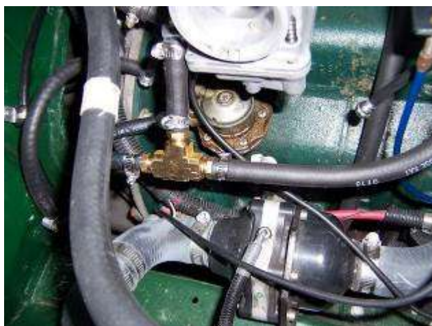
Lowe's special connector for the fuel lines under the rear carb - overkill
