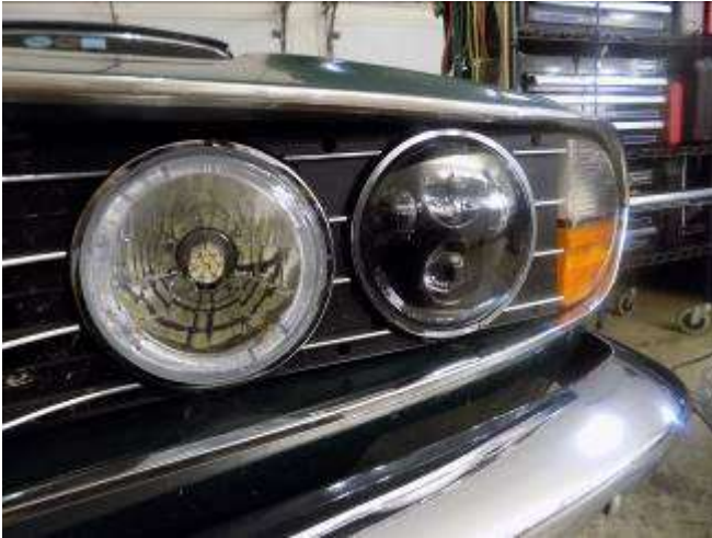
LED headlight mounted and ready to dive – the DRLs are the inner lights, or the one to the left as you look at this
