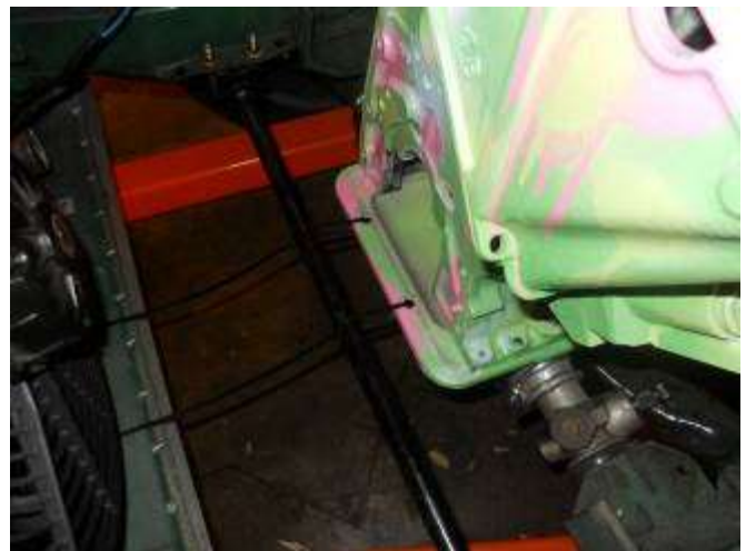
Front engine position located via nylon ties attached to sway bar.
