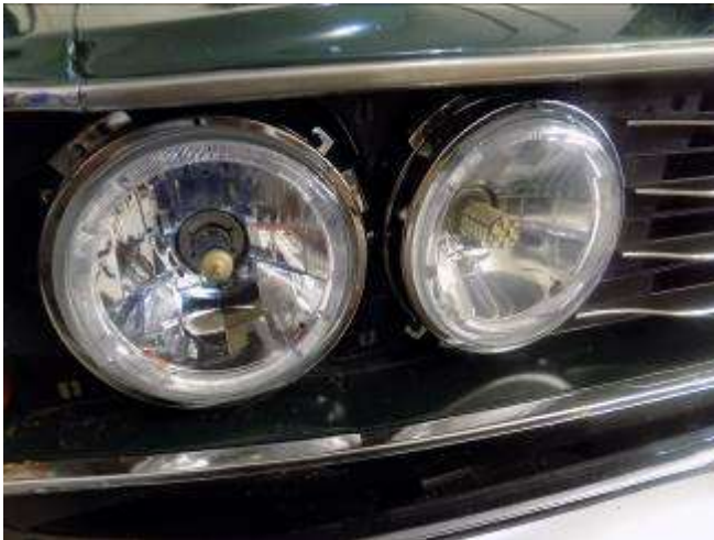
Existing headlights – the one on the left is the “real” headlight using Halogen H4 bulb. The inner ones are daytime running lights now and come on with the ignition
