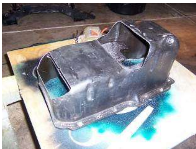
Oil Pan Modified To Clear Front Suspension w/o Lift Kit
