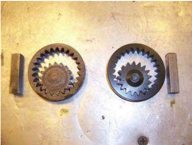
Old Transmission Oil Pump Gear on Left, New One on Right
