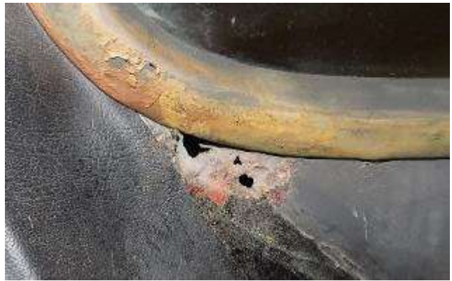
Rust holes under the right side of the windshield
