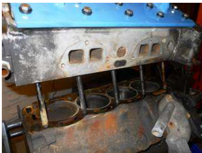
...and off came the head! Check out the corrosion on them studs!
