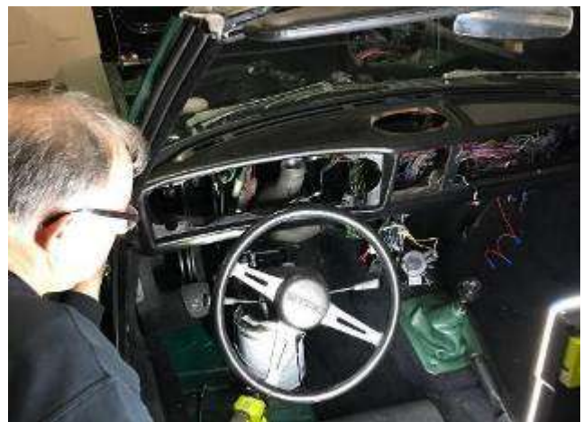
Plexiglas panels out, steering wheel dropped, time to pull the dash! Note the way we put the paint cans to good use.
