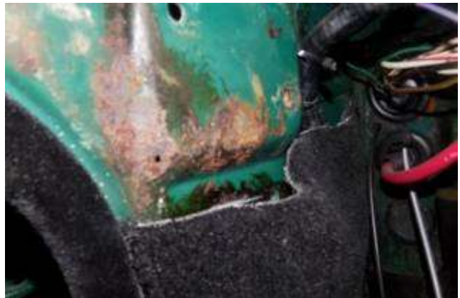
Rust holes a bit further down below where the dash attached due to water coming in the windscreen rubber
