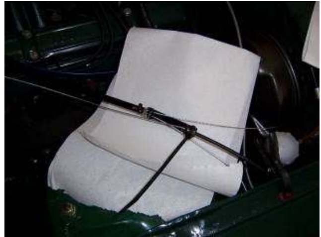
Attaching the choke cables to the CJG – pretty crude, but hopefully workable
