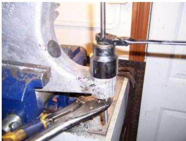
Trailing arm bushing removal tool – large socket is what the bushing presses into from the washer on the threaded rod forcing it up from below – Vise Grip is used to keep rod from spinning
