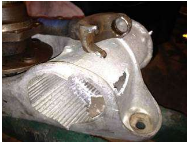
Holes in the trailing arm & busted yoke
