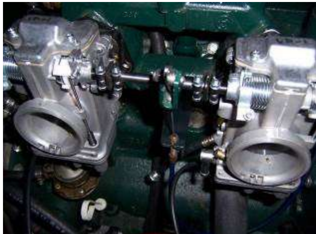
Initial throttle linkage – bracket was made to move the adjuster mounting point farther away from the engine under the shaft
