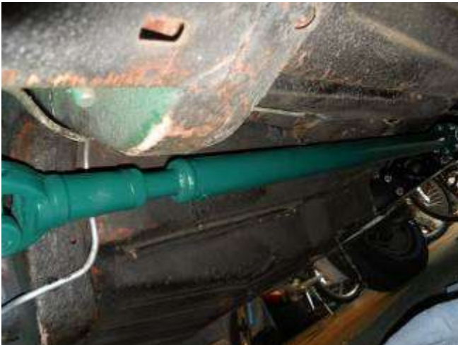
4-Foot Driveshaft. Longest one I've ever seen in a Triumph! We'll see about vibrations...
