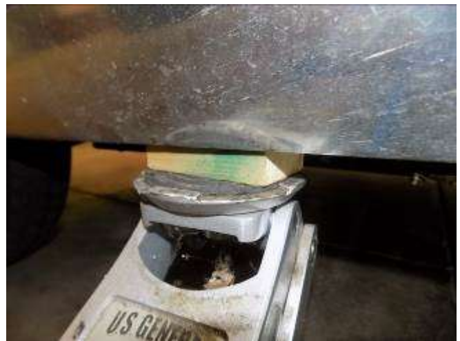
Wood Spacer/locator block in place on the FrankenStag
