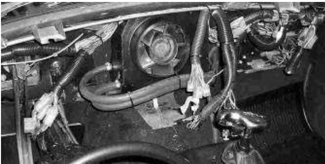
New Heater In Dash Along With rebuilt Wiring Harness – That Was A Lot Of Work!
