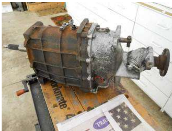
Next Victim – Rover box out of an SD1 that will head into the Stag
