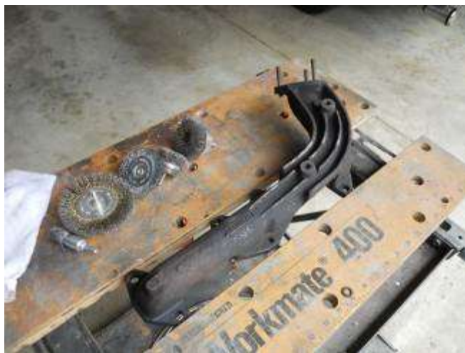
Rust off, ready for first coat
