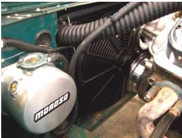
Shot Looking Forward On Drivers Side – Aluminum Expansion Tank And Big Honking Electric Fan
