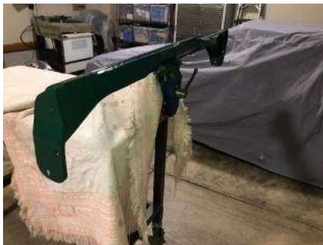
Then the remaining part of the dash had the vinyl and padding ripped off and a coat of green paint attached
