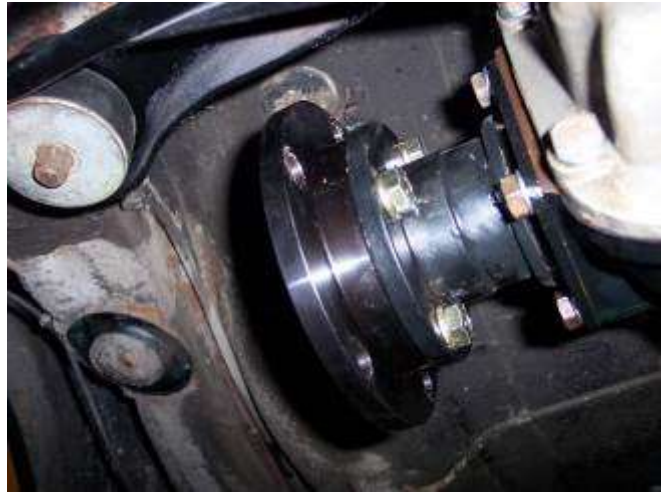
Adaptor plate holding shaft to differential
