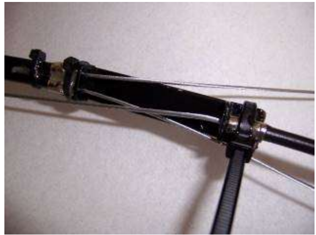
Close-up of the attachment – cables held in place by nylon wire ties and then epoxy put around them. Again, Red Green tips his hat...
