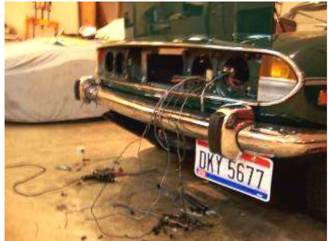
Figure 5: Grille Out, Headlamps Out, Wiring Harness Gutted
