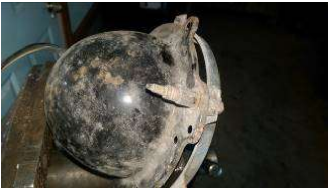
Condition of the adjustors – not too bad, just needed a bit of oil.
