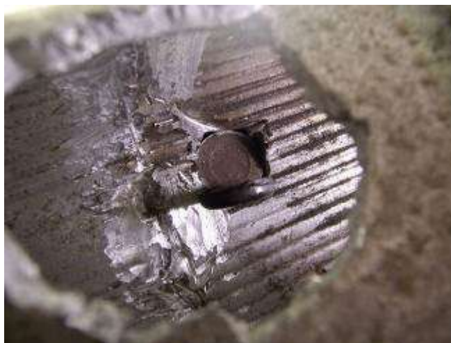
The U-Joint bearing cap embedded in the other side of the trailing arm as seem though one of the holes. Wonderful!
