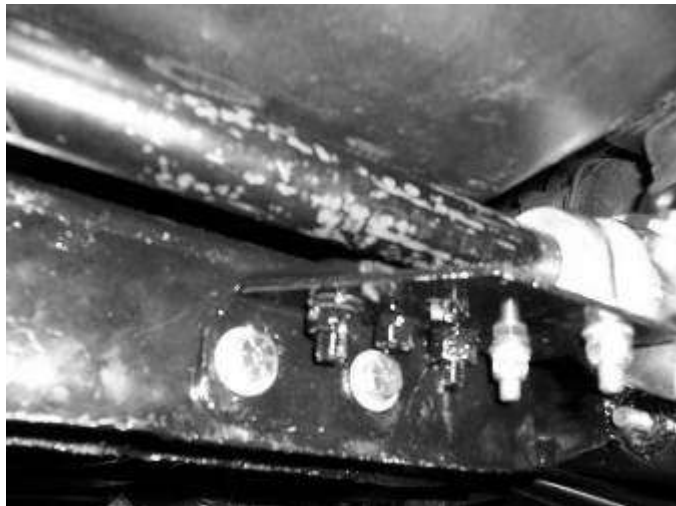
Rack Mount Driver's Side – note close clearance to the oil pan - I got the rack up about as High as I could and engine as low as possible
