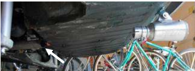
Muffler and pipe in place on the FrankenStag – white arrow shows the end of the pipe that goes through the back sub-frame.
