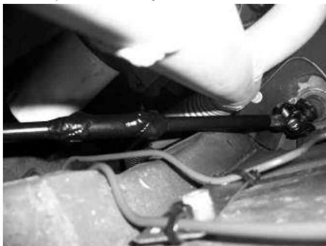
New lower steering shaft in place, fits just right between brake lines and exhaust header.
