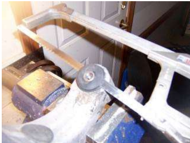
Cutting the protruding part of the bushings off – just use a hacksaw – pretty simple
