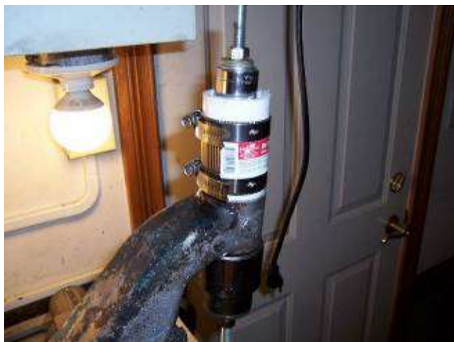
Anti-mushrooming sleeve made from Lowes parts
