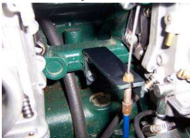
A closer view of the bracket made to hold the throttle cable adjuster
