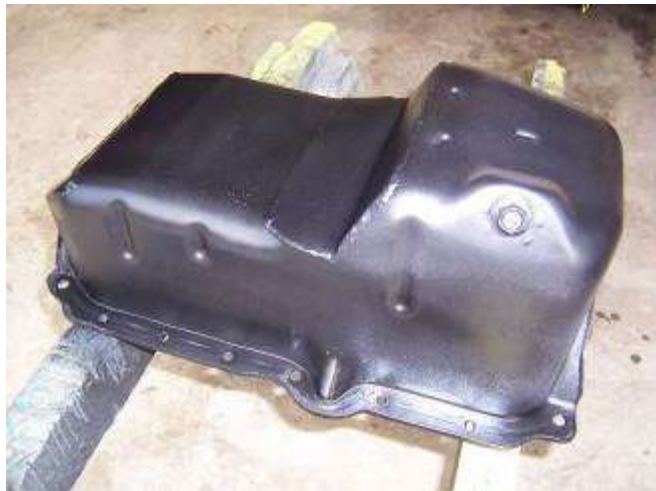
Modified Pan Ready To Put Back On
