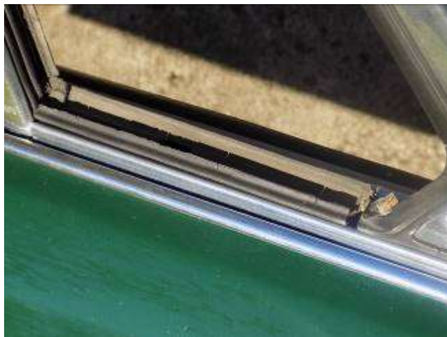
Cracked, broken and HARD quarter seal
