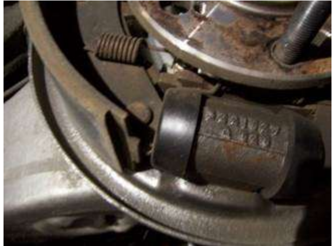
Behind that leading shoe on the driver's side lies the self adjuster that can give you convulsions - patience is the key
