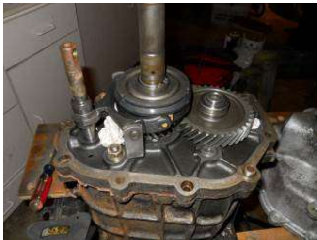
Inside of the back end of the Rover box used in later TR7s and TR8s (and Rover SD's and a few other cars/trucks to boot...) - to the left is the selector shaft. Note the shop rags in the holes in the casting so parts of the gasket I was scraping would not fall in.
