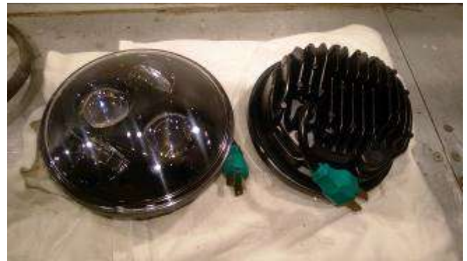
LED bulbs 5.75" Diameter – uses four individual LEDs to produce the light
