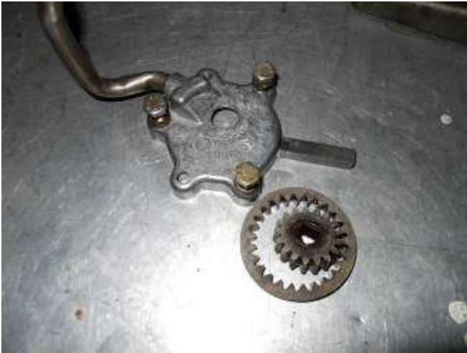
Rover Box Oil Pump – this supplies oil to the rear output shaft bearing. The pump gears are fiber rather than metal, so wear and damage can be a concern.
