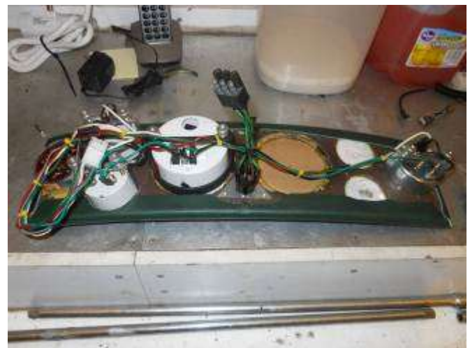
Rewired instrument cluster – added a quick-disconnect for gauge wiring to match the hazard switch and idiot light cluster disconnects – now the whole thing comes off much easier
