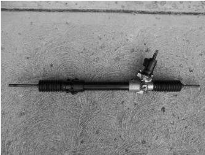
The original Stag Steering Rack modified to be a manual rack – no plumbing!
