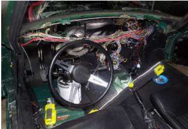
Driver's side - dash out, wired released, steering column still on the paint can...
