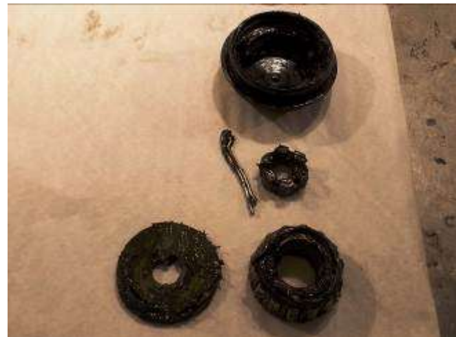
Bearing, D-washer, hub nut, cotter pin, and dust cap as they came off the car
