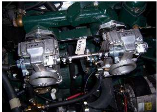
New Mikuni carbs in place on new carb mounts
