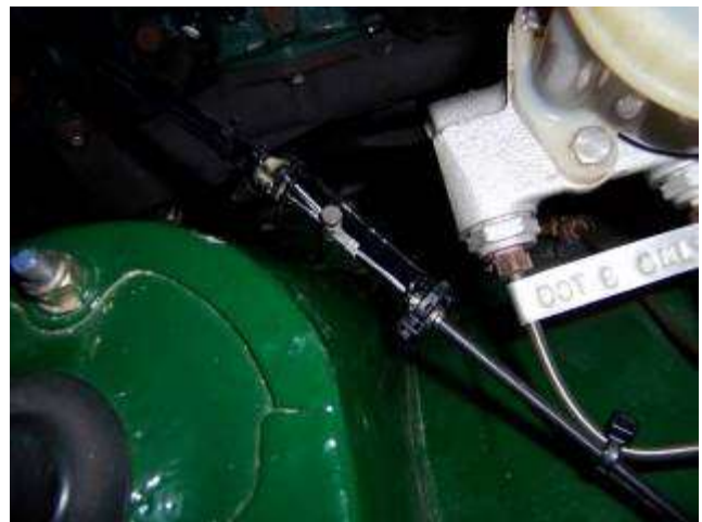
Inside cables soldered, barrel-clamped and in place
