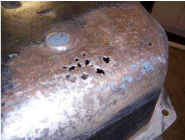
Figure 3: Holes In The Gas Tank
