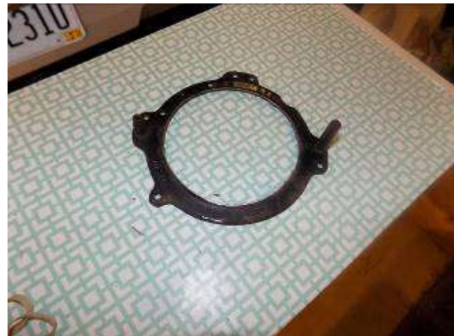
Finished headlight mounting support mount ready for the headlight mounting ring to be attached.
