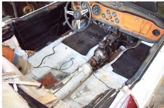
The floor is patched but still has two fasteners rusted in place. I twisted the heads off. I need to remember that this is not a Ford. Fine threads and they are a bit fragile in comparison.
