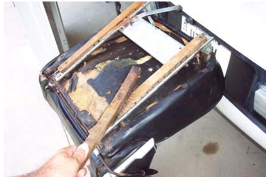
Wire brush strokes loosen the rust before applying chemicals or paint.
