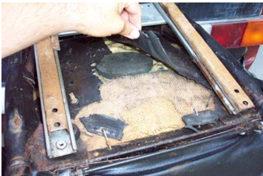
Tragic result of rubber products in seat bottom deteriorating over time and use. This lets my bumm down into an uncomfortable depression between hard seat sides. It must go.
