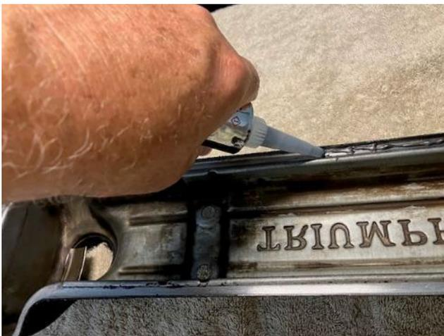
**Running a small bead of black silicone valve cover sealer around the edge**
