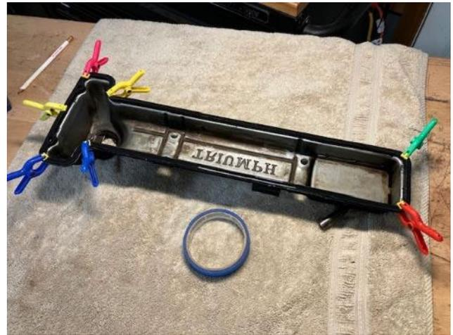
**Clamped into place while the sealant cures**
