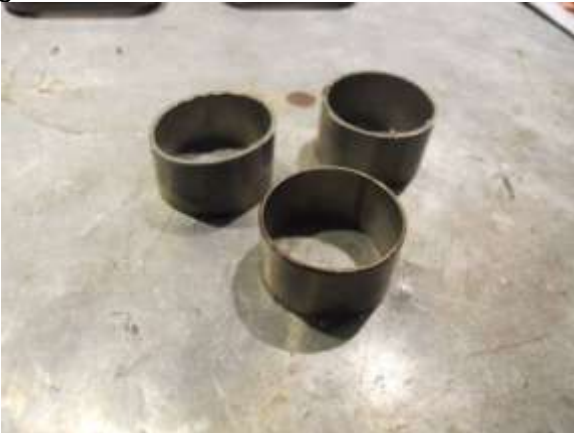
Excess length that came off the radiator pipe
