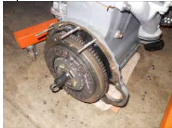
Clutch disc in place ready for fitting the pressure plate assembly – note the guide rods in place above the flywheel
