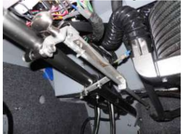
Choke mechanism mounted on the steering column
