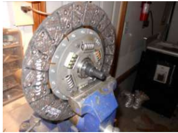
In the process of filing away the front (rearward) part of the clutch plate splines – checking fit with the alignment tool
