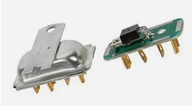
Vendor picture of the guts inside Chuck's failed regulator – note no capacitors and no real heat sinking, the regulator is just bent over so it fits in the "can"
