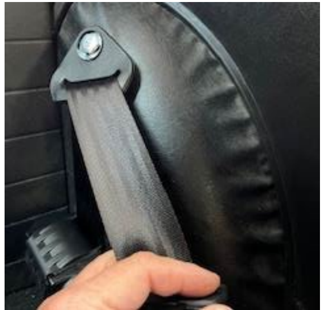
New guide in position using the same mounting point as the original
