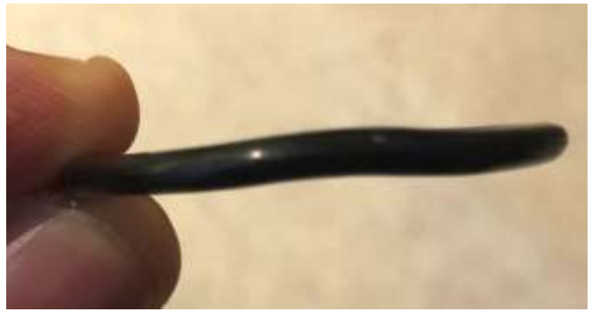
Flattened and wavy...not how I like my O-Rings...
