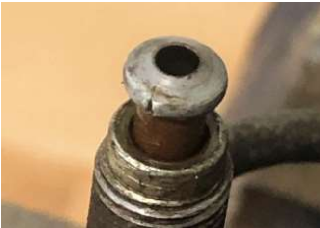
Flattened and cracked brake line end flare - not for reuse!
