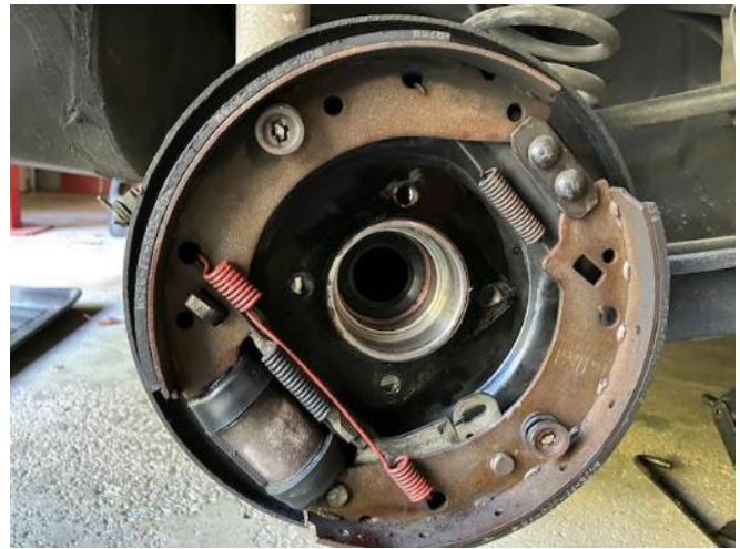
New inner oil seal in place
