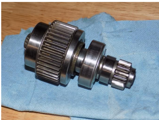
Aftermarket High Torque Starter Drive Assembly
