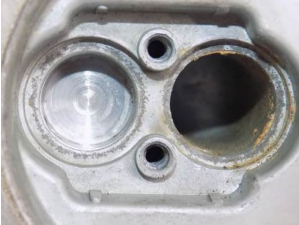
Early, Mid, and some Late AC pumps used a clip to hold in inlet/outlet valves
