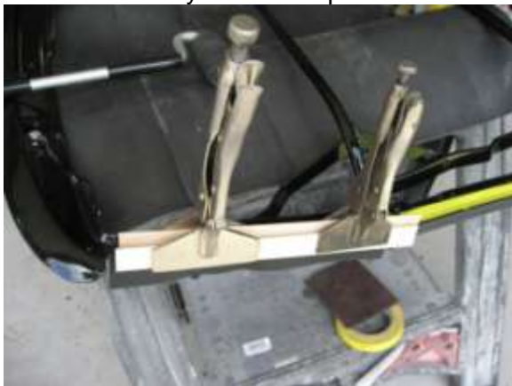
The strips I got from TRF had Velcro that was 1" wide. The area that the Velcro covers is 5/8" wide. This would have made an unsightly install in my opinion so I took the strips to a local upholsterer and he cut one of the seams and trimmed 3/8" off the Velcro and sewed them back on. Much better.
