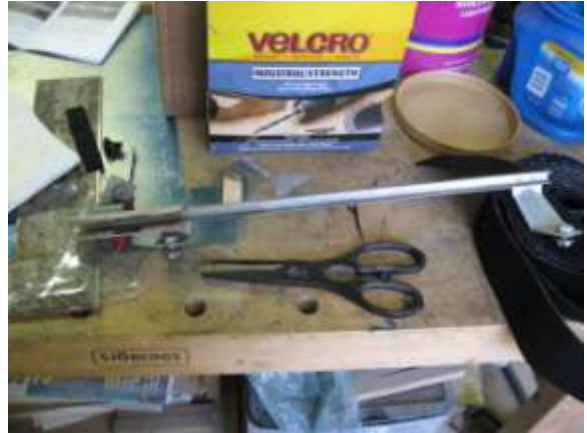
I then placed the Velcro on the edge of the window which I clamped in a vise and then forced the rail down over it.
