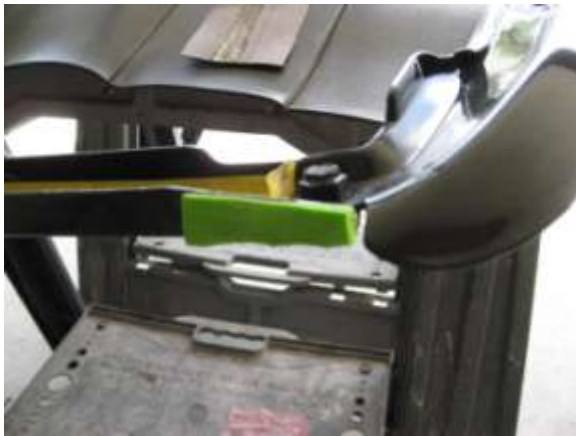
After roughing up the area I applied contact cement and used strips of wood and clamps to attach the vinyl/Velcro strips.
